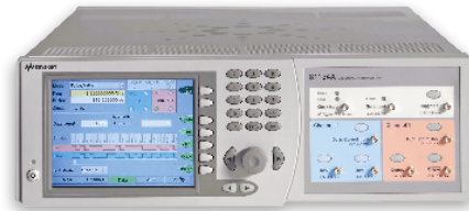
Keysight 81134A | 脈衝圖形生成器; 2通道, 3.35GHz
