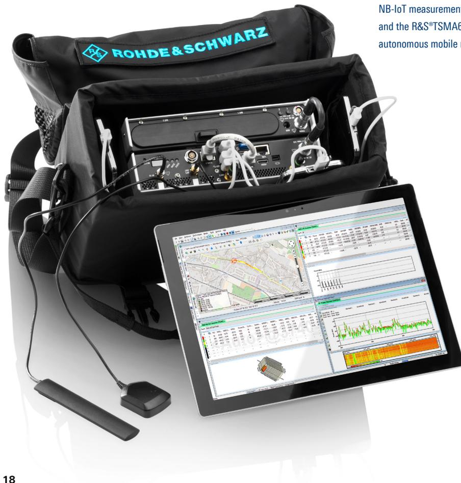
NB-IoT measurements with R&S®ROMES4 and the R&S®TSMAG/R&S®TSMA6B autonomous mobile network scanner.
