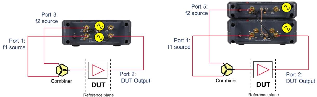
Configuration using a 4-port P502xA (left), 6-port configuration using 2-port P500xA and 4-port P502xA (right).
