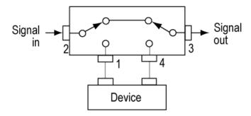
Figure 5. Keysight 8763 used as a transfer switch (equivalent circuit action)
