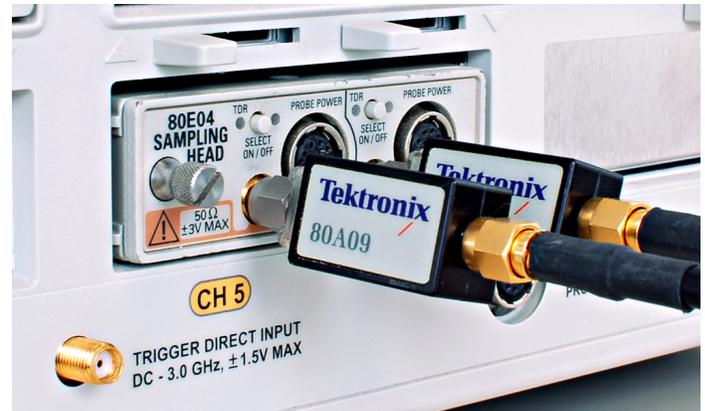
Sampling modules with dual electrical channels, such as the 80E04 dual-channel 20 GHz electrical sampling module with TDR, require two 80A09 devices. Step generators within the 80E04 TDR modules uses  $\leq 250$  mV, which is less than the diode threshold of the 80A09 device.
