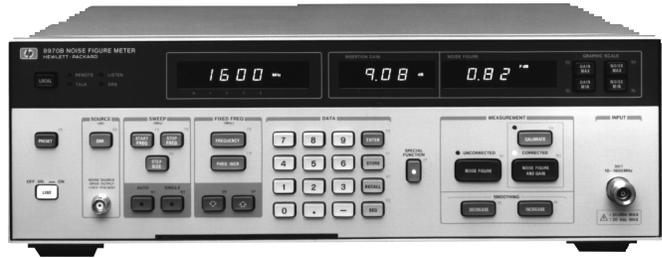
HP 8970B Noise Figure Meter (10 to 1600 MHz).
