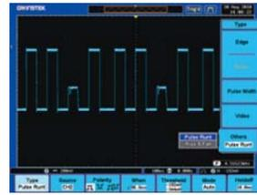
Besides Edge trigger, the GDS-3000 Series also offers various trigger functions, including Video, Pulse Width, Runt, Rise Time & Fall Time (specific time length), Alternate, Delay by Time, Delay by Event, and Hold-Off. The high sampling rate, the VPO signal processing & display, and the flexible trigger function all together make the GDS-3000 Series a powerful tool for waveform capture and display of various types of signals.
