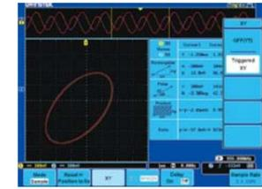
The X-Y mode of GDS-3000 defines CH1 and CH3 as the horizontal axis and CH2 and CH4 as the vertical axis, allowing the display of 2 sets of X-Y pattern simultaneously. The measurement items include Rectangular, Polar, Product and Ratio that fits most of the popular X-Y applications. The X-Y pattern and the time domain waveforms can be shown on the screen simultaneously. Two cursors on the time domain waveforms allow the identification of cursor-associated locations on the X-Y pattern display.
