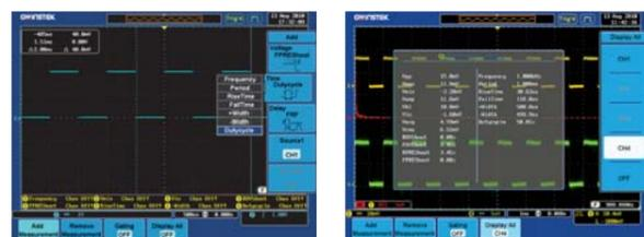
The GDS-3000 Series supports simultaneous measurement of up to 28 waveform measurement items grouped into three main waveform parameters: amplitude, time and delay measurements. The display modes include an individual mode and a Display All mode. The former can display any 8 of the automatic measurements while the later can display all the automatic measurements for a channel.
