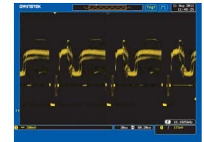
The GDS-3000 Series equipped with VPO signal processing technology and 5GSa/s high-speed real-time sampling rate, allows you to view the video signal clearly.
