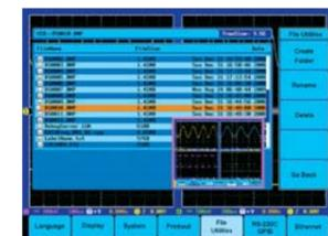
The GDS-3000 provides an optimized operation interface for viewing screen captures. Generally, the oscilloscope may store large amounts of waveform data after a long period of time. To help prevent engineers from selecting the wrong file from a large number of stored waveform files, the screen capture preview function can be used to preview the waveform file without opening files so that operation of the oscilloscope is more efficient and convenient.
