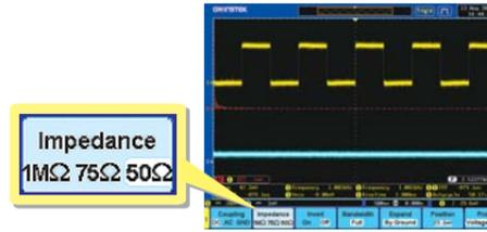
Three input impedance, 1MΩ, 75Ω, and 50Ω are available for user's selection. The flexibility of impedance selections, including 1MΩ to get minimum loading effect, 75Ω to accommodate Video transmission applications and 50Ω to fit RF communication applications, extends the GDS-3000 Series utilization range.
