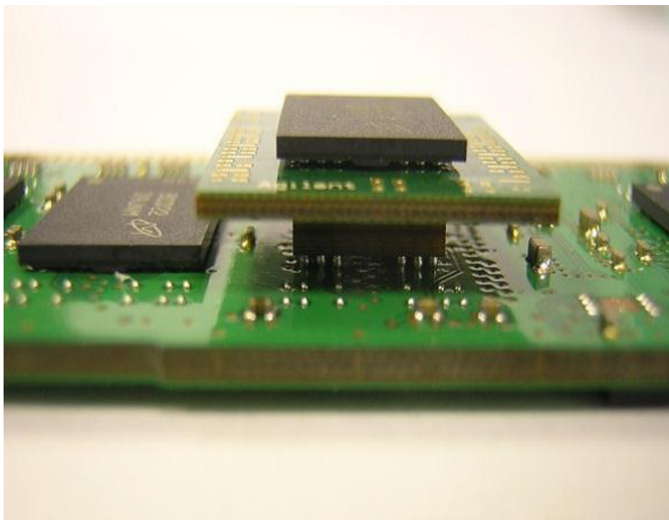
Figure 1. Photo of stacked DIMM-Riser-Interposer-DDR.
