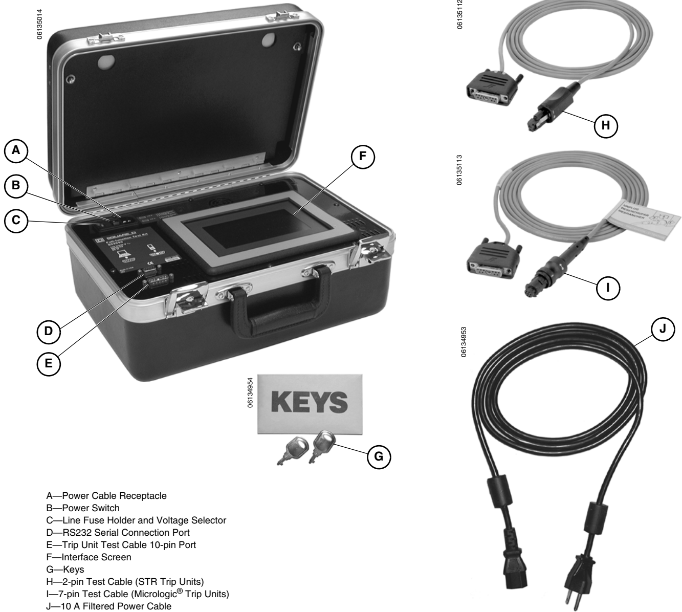
Figure 1: Full-function Test Kit and Case Contents
