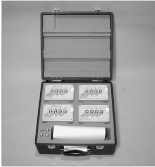
**Terminal Connector:** 4-Terminal Pair, BNC
