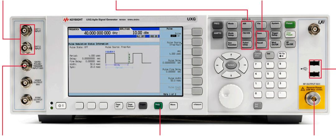
Accept input signals for external pulse modulation with Gate/Pulse/Trigger input (Option PM1).
