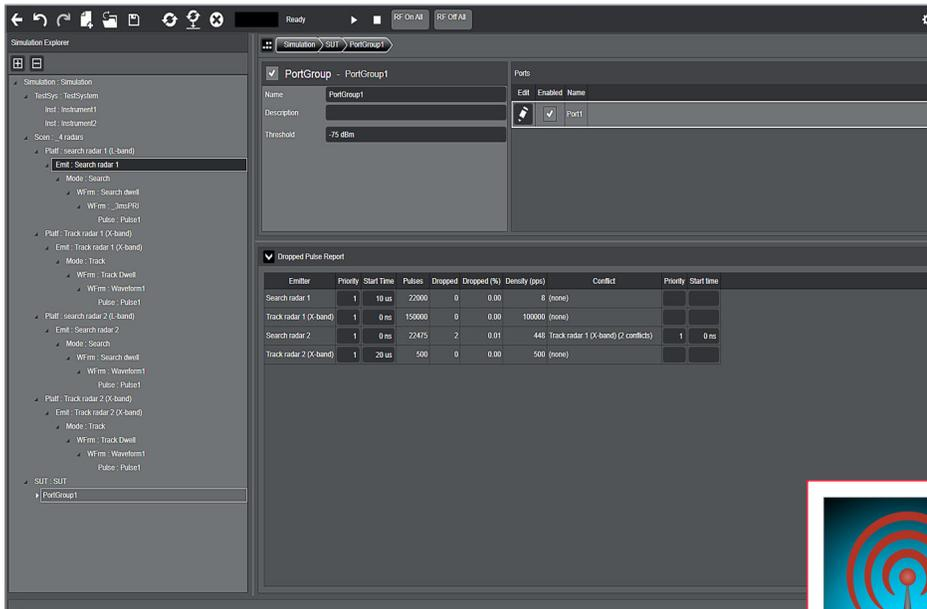
The screenshot displays the Signal Studio software interface. On the left is a 'Simulation Explorer' tree showing a hierarchy of components including 'TestSys - TestSystem', 'Incident1', 'Incident2', 'Scan - 4 radars', and 'SUT - SUT'. The main area shows the configuration for 'PortGroup1', including a 'Ports' table with 'Port1' selected. Below this is a 'Dropped Pulse Report' table with the following data:
