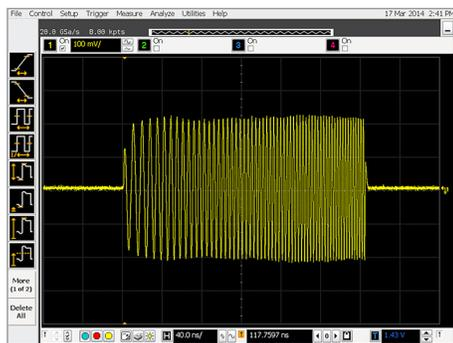
Generate wide chirps that are 10 to 25 percent of carrier frequency
