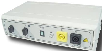
Solid-state switch for energizing loads (up to 200Apk) at either the peak or the zero crossing of AC voltage. Ideal for inrush current testing.
