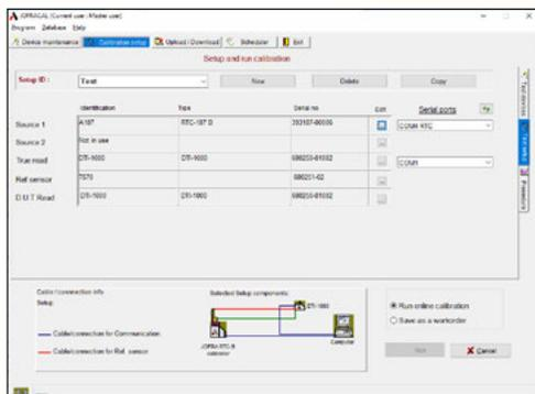
JofraCal is a highly versatile calibration software that is supplied together with the RTC calibrators. The software ensures easy calibration of all kinds of temperature sensors, such as RTD's, thermocouples, transmitters, and thermoswites. Furthermore, it can be used for pressure calibration i.e. pressure gauges and pressure switches. JofraCal integrates with Jofra calibration instruments. As for temperature calibrators, it is the whole range
