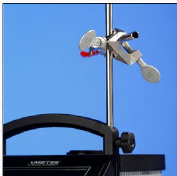
The integrated support rod is part of the reduced weight philosophy. It is lightweight and very easy to mount on the RTC. Two fixing holes are integrated in the calibrator where the support rods can be mounted.
