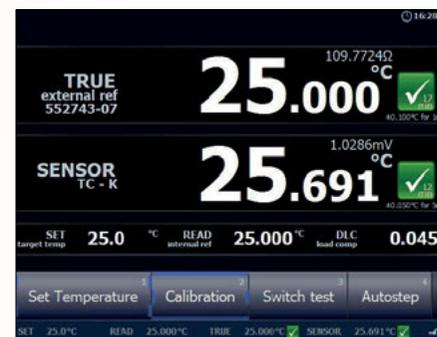
Model B of the RTC is equipped with a built-in accurate measuring circuit for sensor-under-test (input), which enables measurement of virtually any type of temperature sensors including: Resistance thermometers (RTD), thermocouples (TC), transmitters, milliamps (mA), voltage (V) and thermostats.
