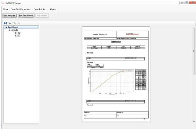
PDF test report from determine the knee point voltage of the current transformer.
