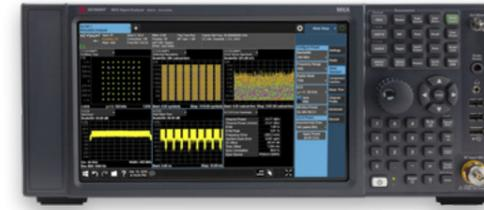
**Keysight N9021B** | MXA Signal Analyzer; 10 Hz to 50 GHz
