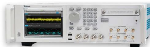
**Tektronix AWG70002B** | Arbitrary Waveform Generator; 2 Channels at 25 Gs/s
