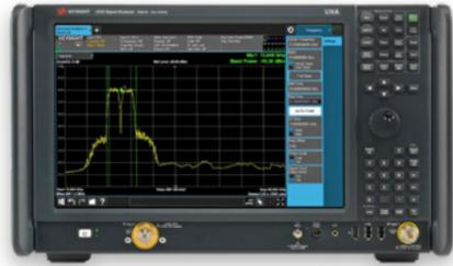
**Keysight N9041B** | UX Signal Analyzer; 2 Hz to 110 GHz
