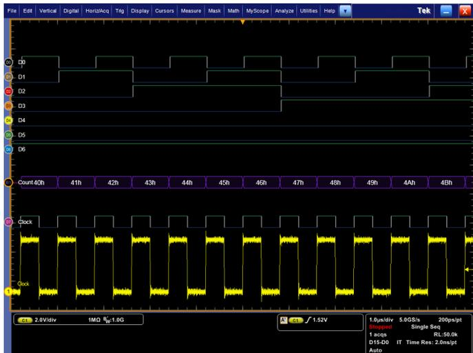
With the color-coded digital waveform display, low values are shown in blue and high values are shown in green, enabling instant understanding of the bus value whether transitions are visible or not. You can set threshold values for each channel, enabling support for up to 16 different logic families.
