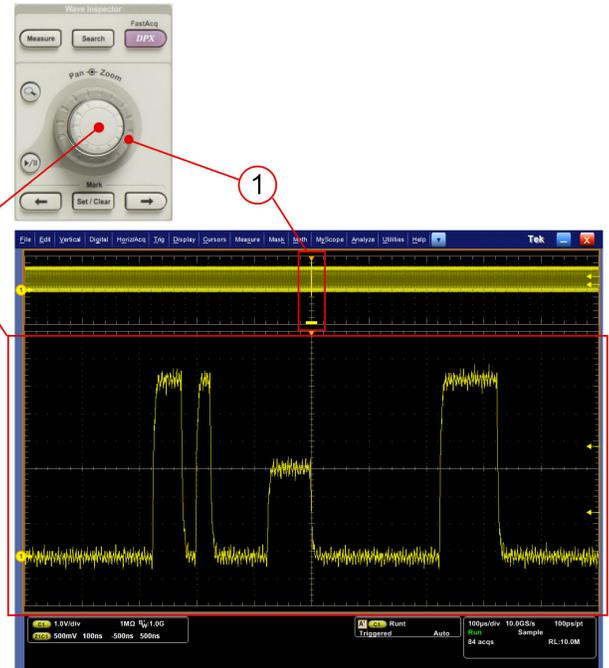
Wave Inspector controls provide unprecedented efficiency in viewing, navigating, and analyzing waveform data. Zip through your long record by turning the outer pan control (1). Get from the beginning to end in seconds. See something of interest and want to see more details? Just turn the inner zoom control (2).
