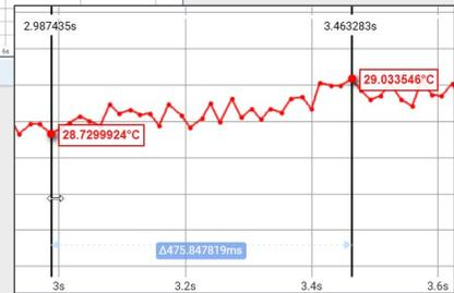
Use cursors to get information on multiple data series or to calculate differences on the horizontal scale.
