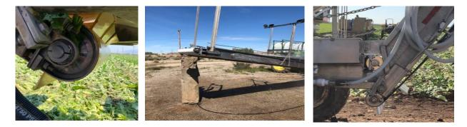
Remove or slacken belt; swab roller and bearing/bushing
