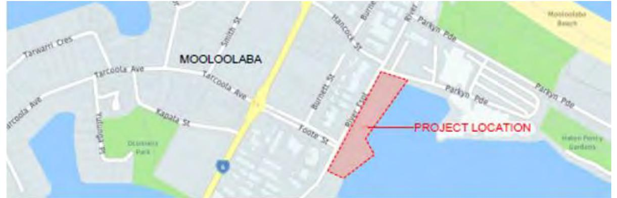
Design has commenced to rebuild the dilapidated rock seawall bounding the park and sea channel to the marina. A new footpath and balustrade will be installed running along the edge of the new seawall.
