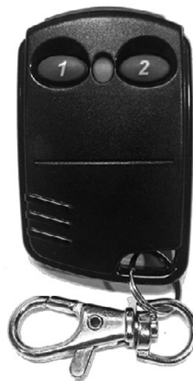
Figure 1: Parrearra Lock wireless remote (FOB) note: both buttons will operate the lock
