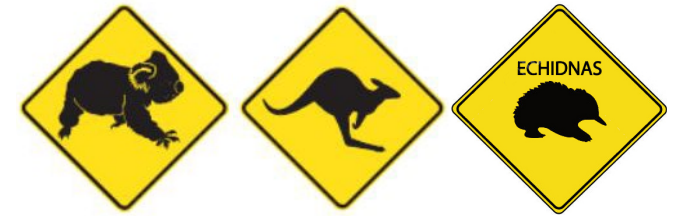
Figure 7: MUTCD wildlife warning road signs (not to scale – for guidance only – site specific design required)
