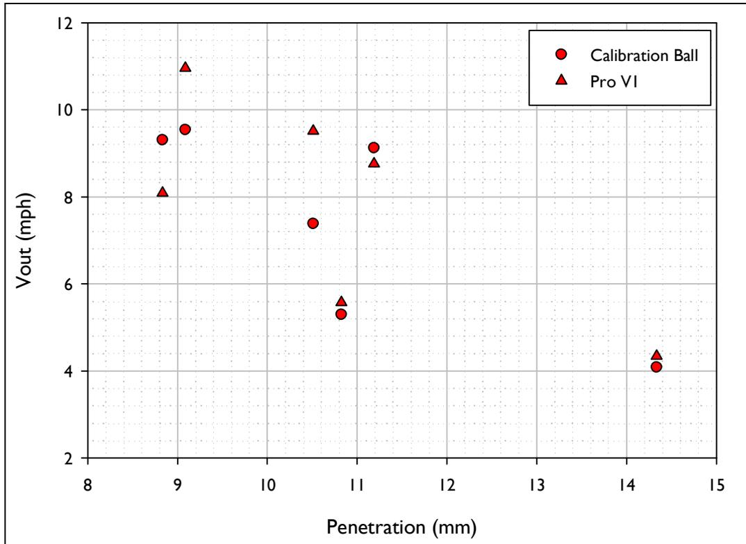
Figure G.1. Outbound speed (Vout) vs. Penetration for the shots fired using the inbound conditions akin to those for a Sand Wedge.
