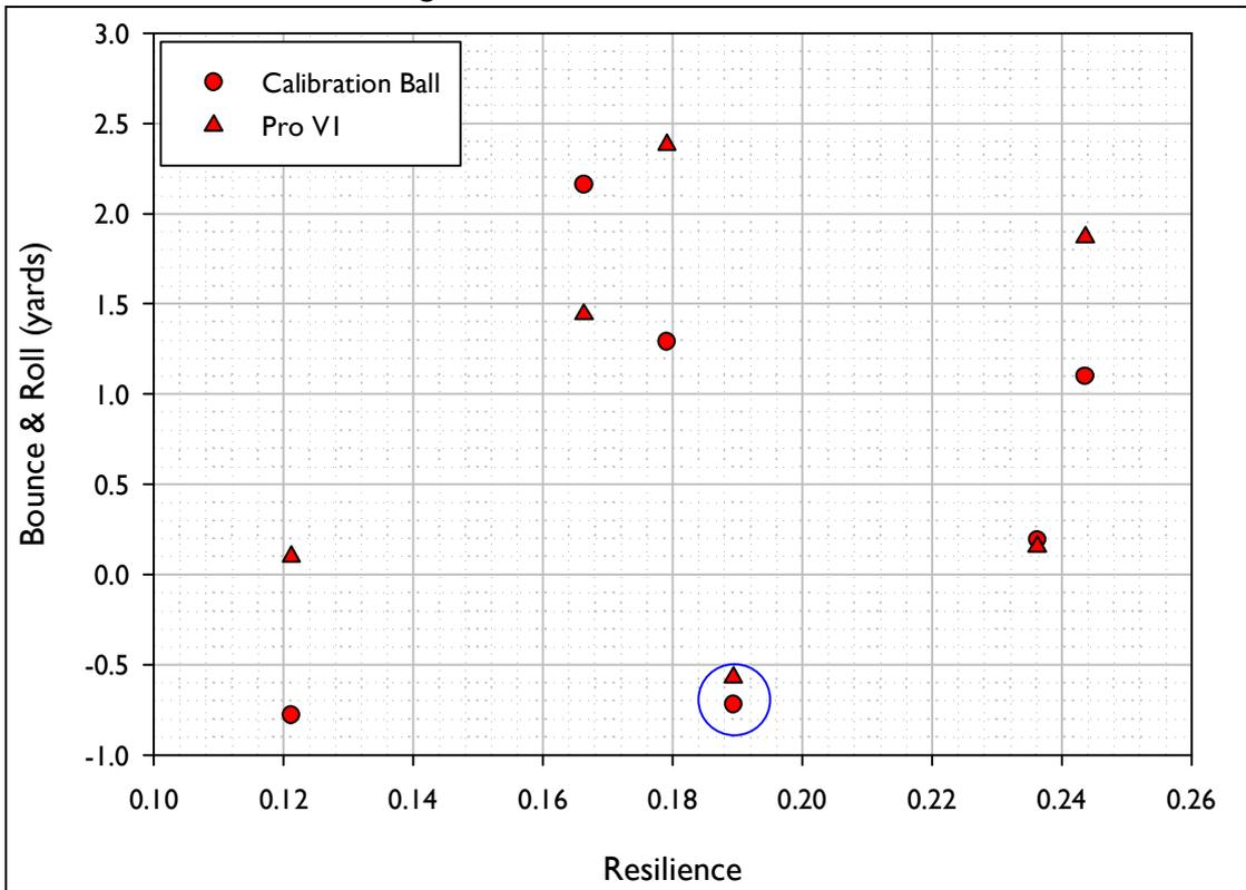
Figure 42. Bounce & Roll vs. Resilience for the shots fired using the inbound conditions akin to those for a sand wedge.
