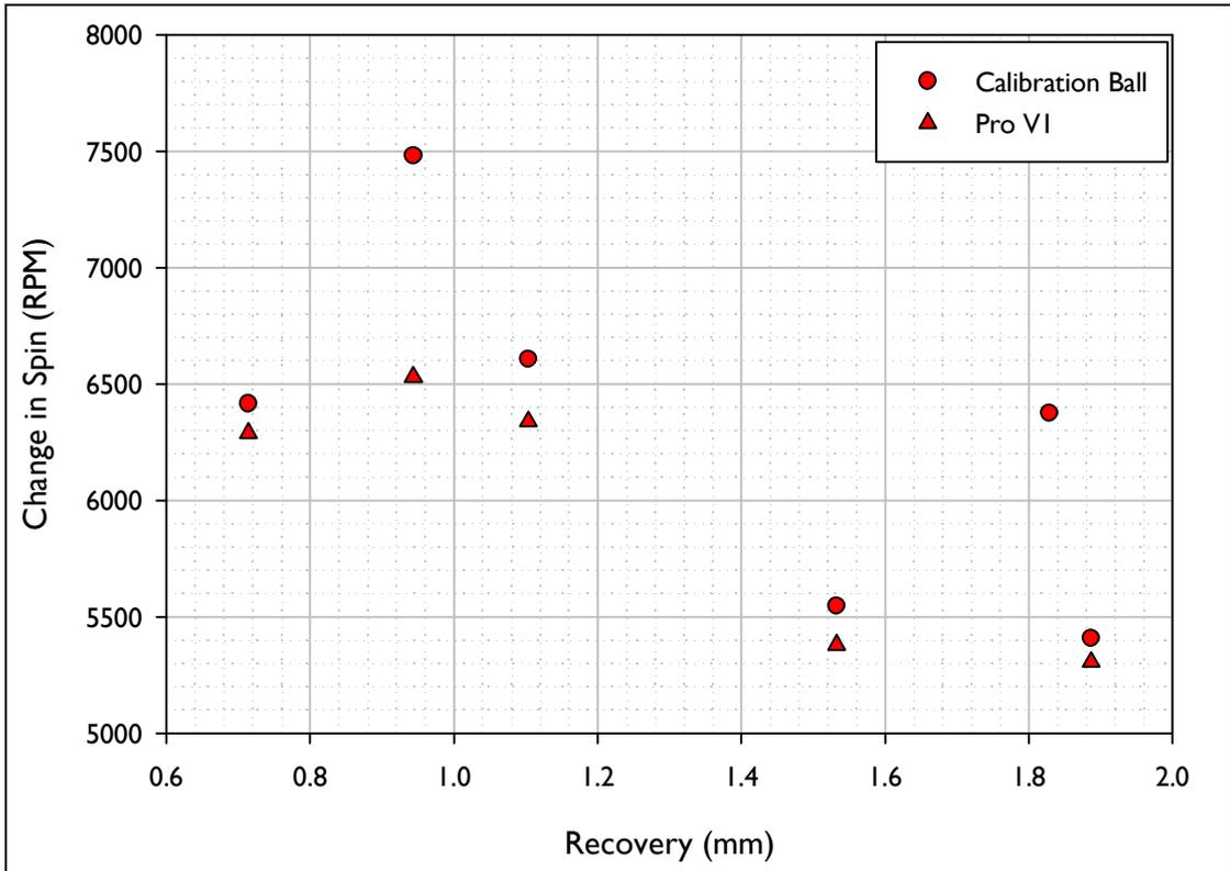
Figure E.3. Change in Spin vs. Recovery for the shots fired using the inbound conditions akin to those for a 5 Iron.
