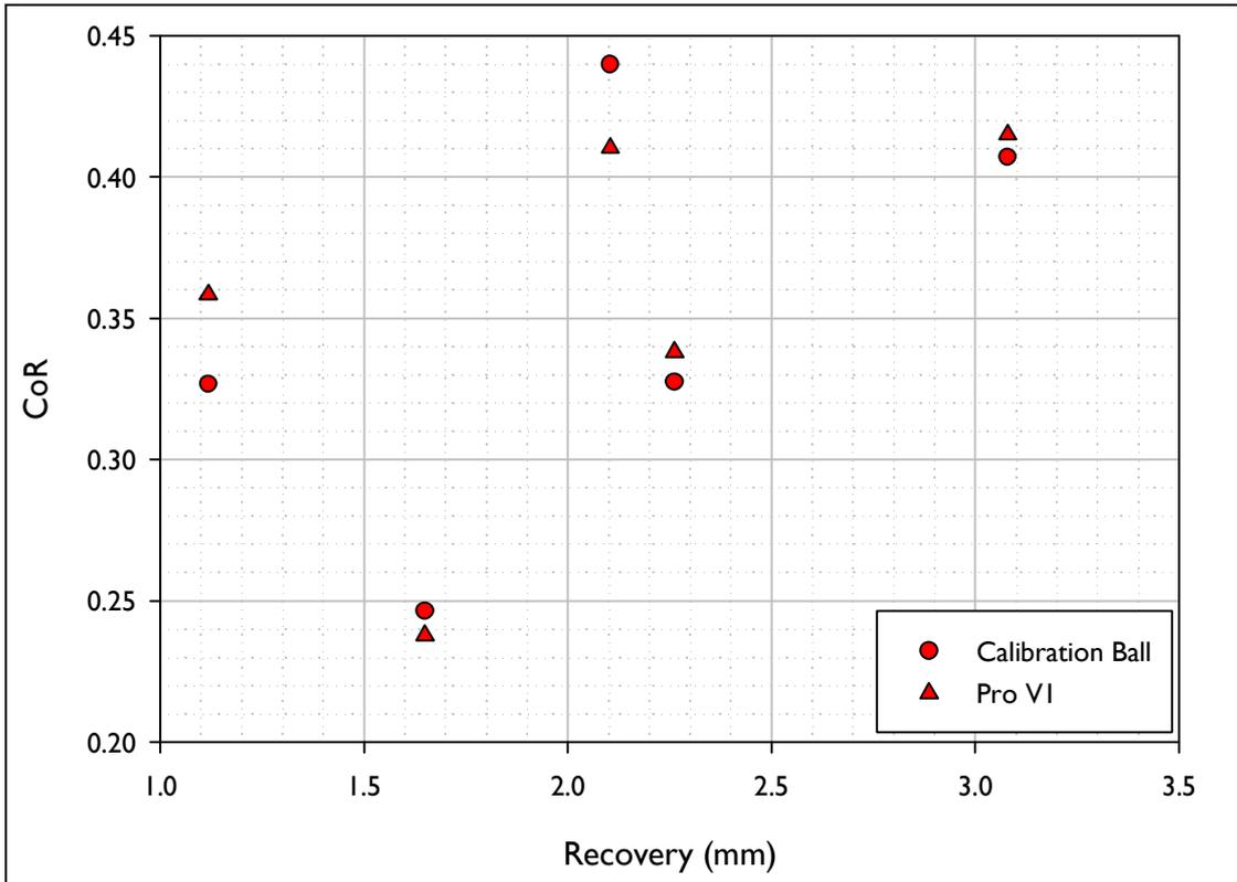
Figure B.5. Vertical Coefficient of Restitution (CoR) vs. Recovery for the shots fired using the inbound conditions akin to those for a Driver.
