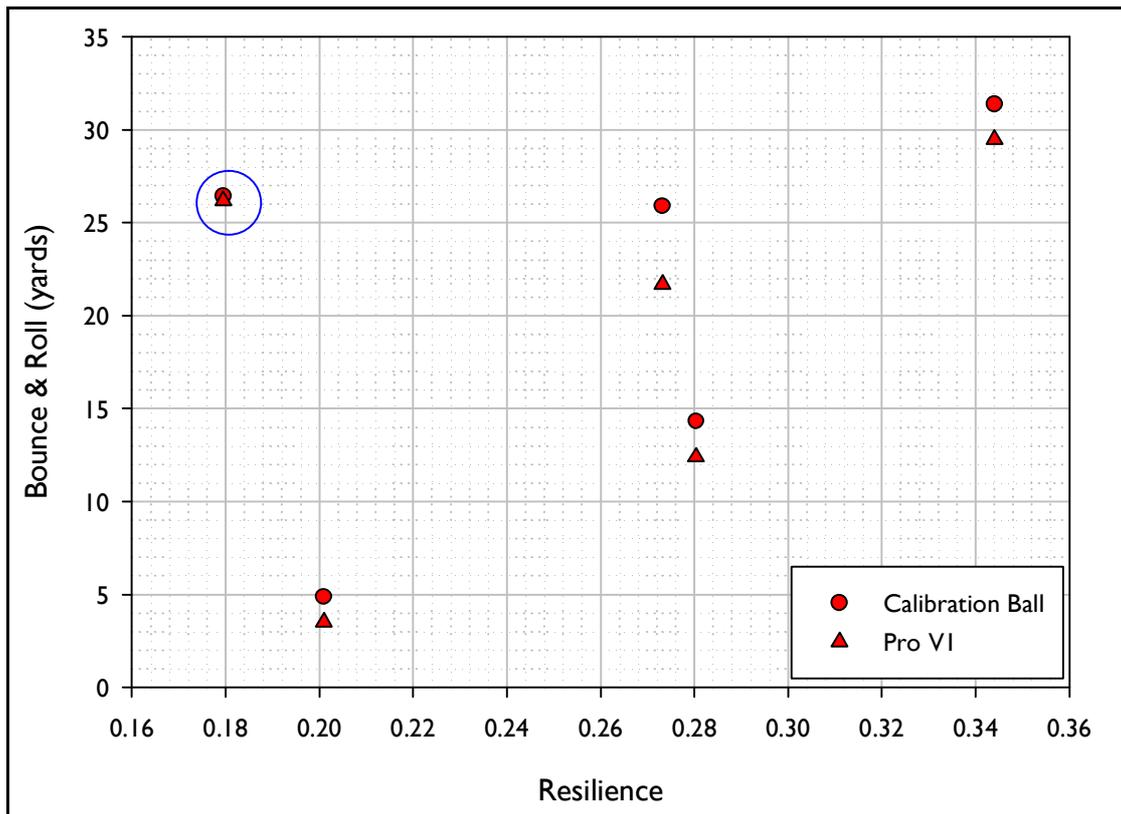
Figure 18. Bounce & Roll vs. Resilience for the shots fired using the inbound conditions akin to those for a Driver.
