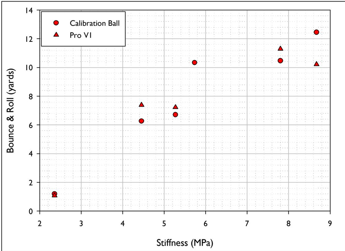
Figure 29. Bounce & Roll vs. Stiffness for the shots fired using the inbound conditions akin to those for a 5 Iron.
