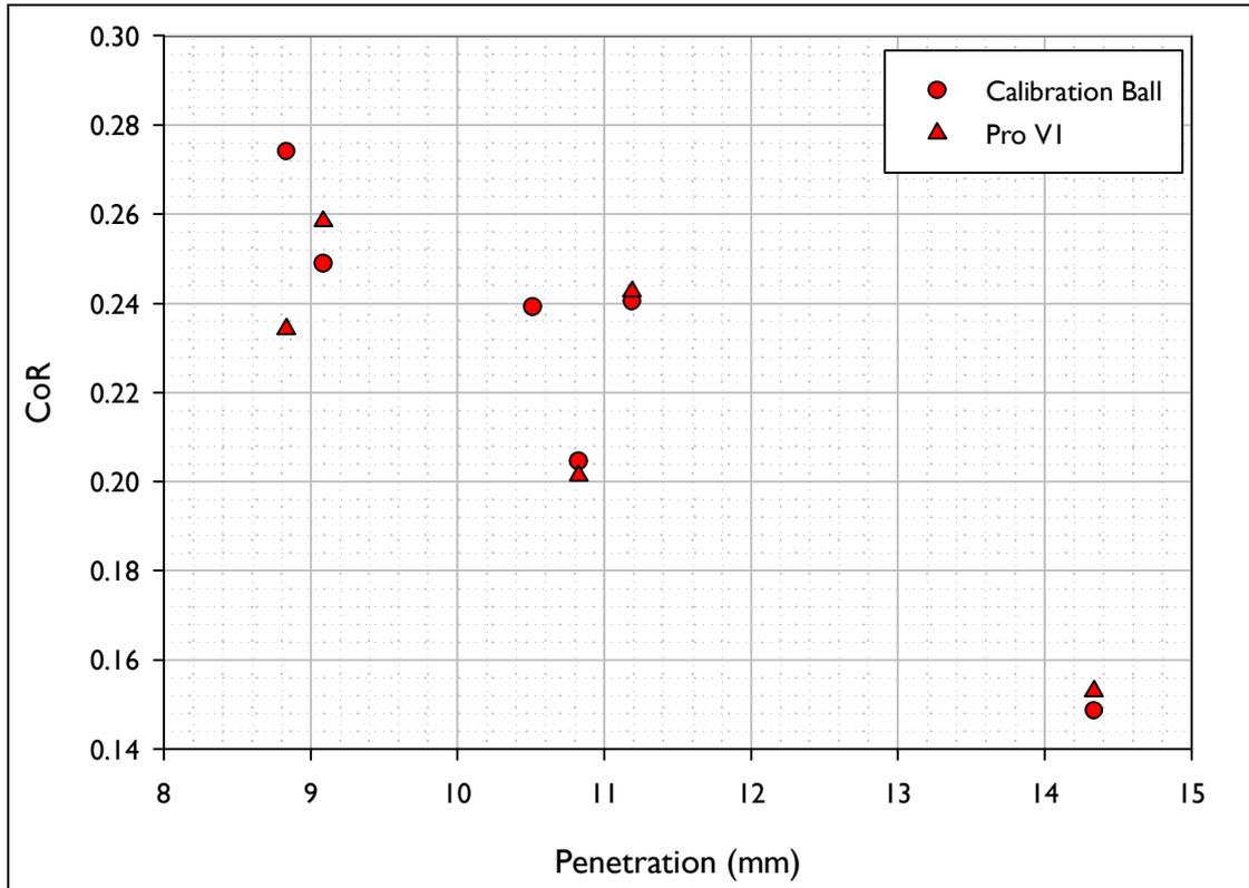
Figure D.5. Vertical Coefficient of Restitution (CoR) vs. Penetration for the shots fired using the inbound conditions akin to those for a 5 Iron.
