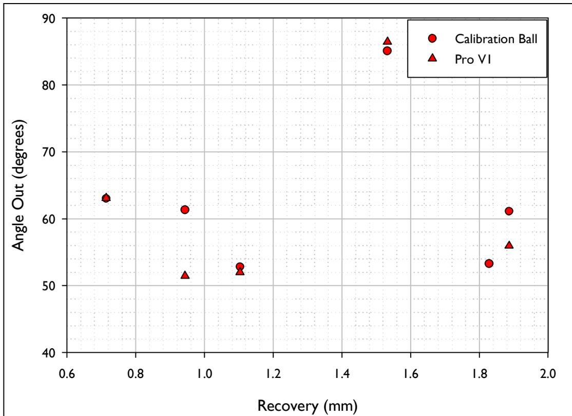
Figure E.2. Outbound Angle after Impact vs. Recovery for the shots fired using the inbound conditions akin to those for a 5 Iron.
