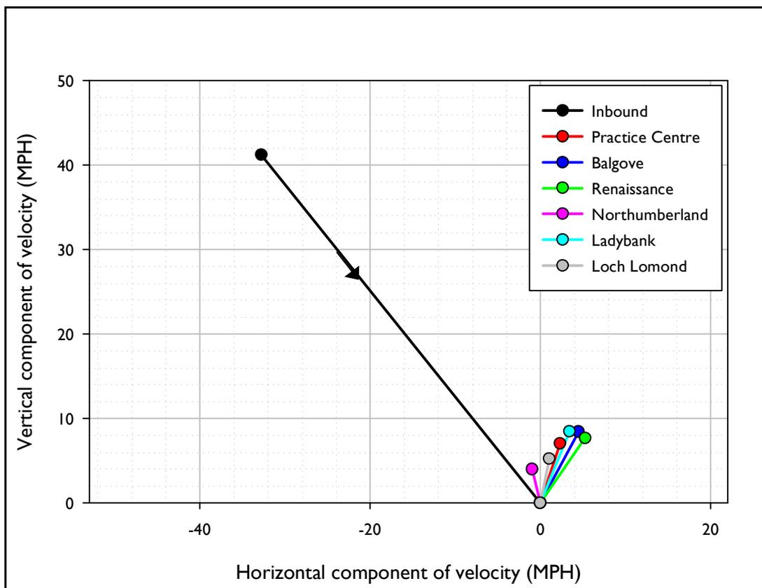
Figure 34. Inbound and Outbound velocity vectors for the Calibration ball when launched with sand wedge impact conditions.
