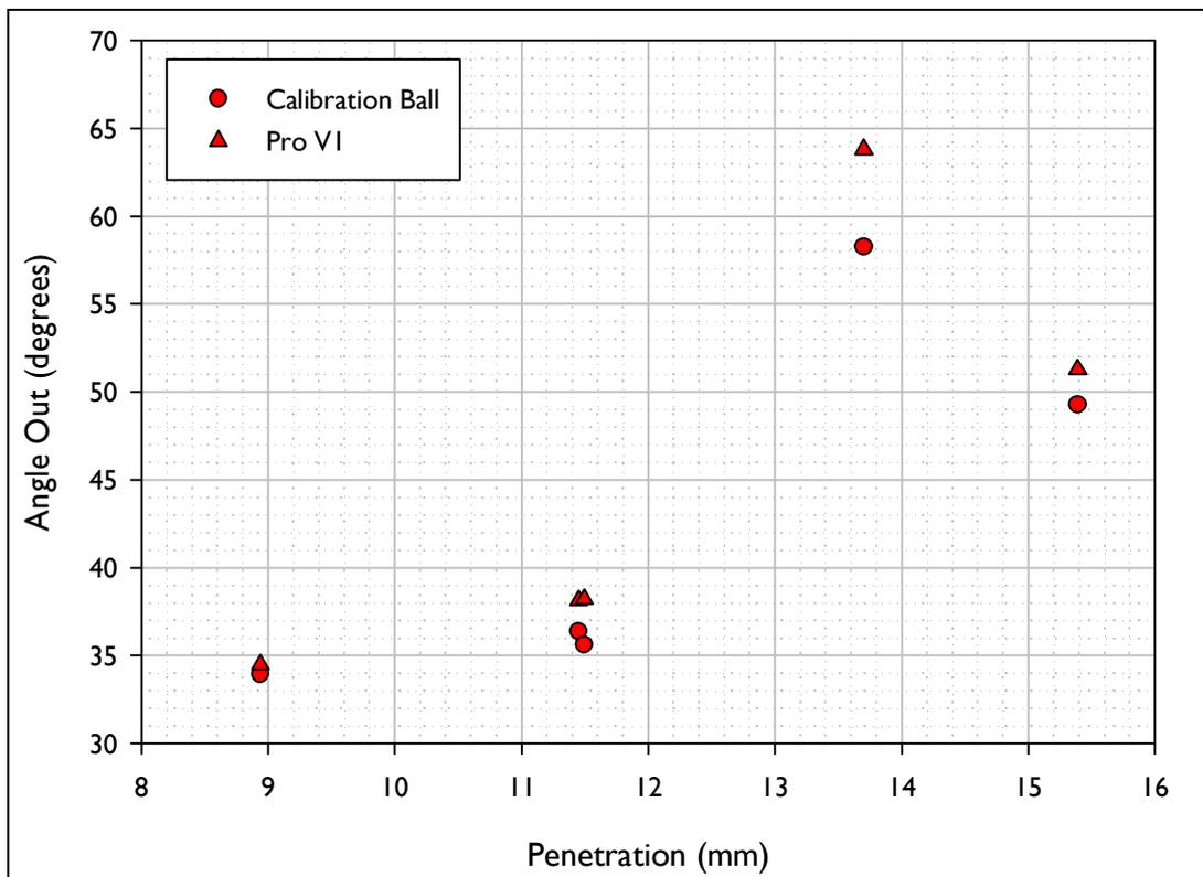
Figure A.2. Outbound Angle after Impact vs. Penetration for the shots fired using the inbound conditions akin to those for a Driver.
