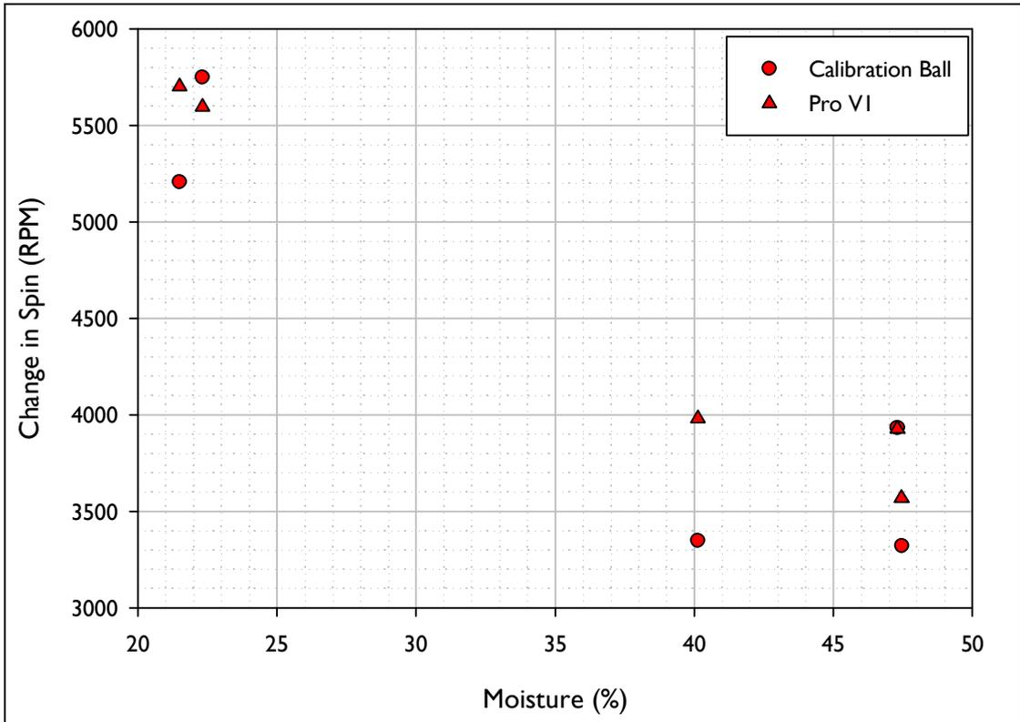
Figure C.3. Change in Spin vs. Moisture for the shots fired using the inbound conditions akin to those for a Driver.
