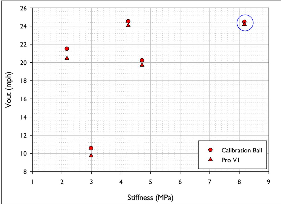
Figure 11. Outbound speed (Vout) vs. Stiffness for the shots fired using the inbound conditions akin to those for a Driver.
