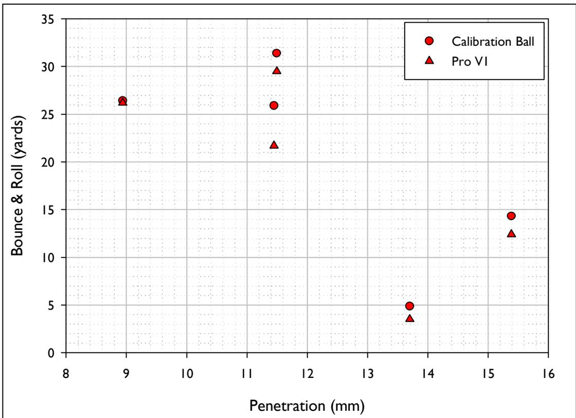
Figure A.4. Bounce & Roll vs. Penetration for the shots fired using the inbound conditions akin to those for a Driver.
