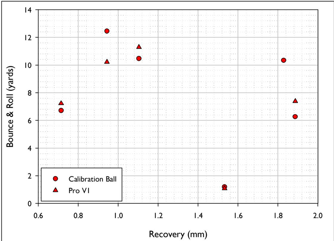
Figure E.4. Bounce & Roll vs. Recovery for the shots fired using the inbound conditions akin to those for a 5 Iron.
