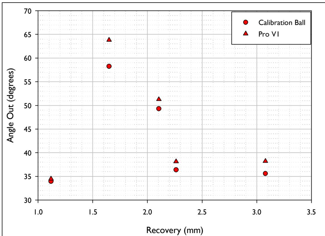
Figure B.2. Outbound Angle after Impact vs. Recovery for the shots fired using the inbound conditions akin to those for a Driver.
