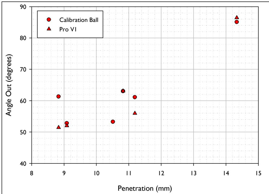
Figure D.2. Outbound Angle after Impact vs. Penetration for the shots fired using the inbound conditions akin to those for a 5 Iron.
