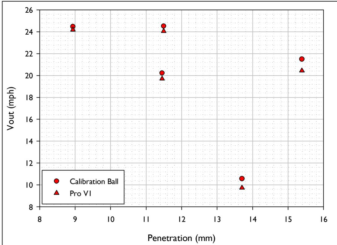
Figure A.1. Outbound speed (Vout) vs. Penetration for the shots fired using the inbound conditions akin to those for a Driver.
