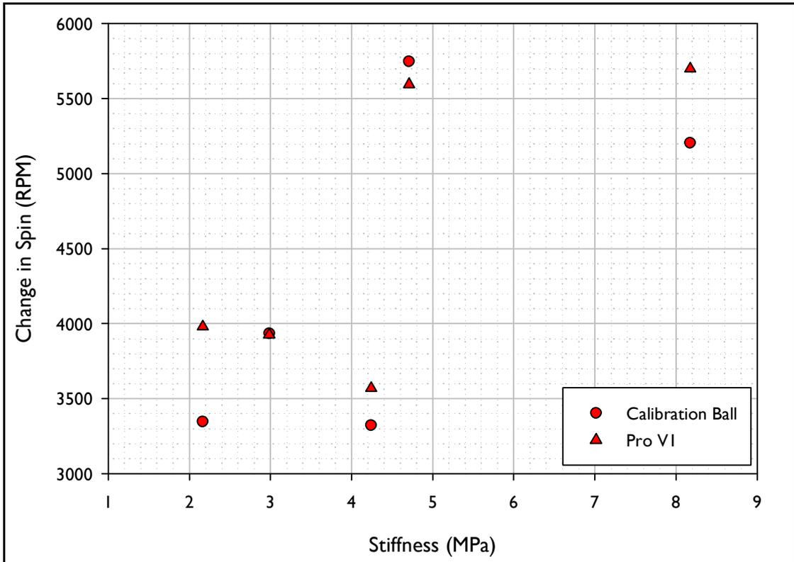
Figure 15. Change in Spin vs. Stiffness for the shots fired using the inbound conditions akin to those for a Driver.
