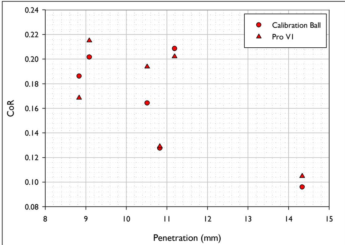
Figure G.5. Vertical Coefficient of Restitution (CoR) vs. Penetration for the shots fired using the inbound conditions akin to those for a Sand Wedge.
