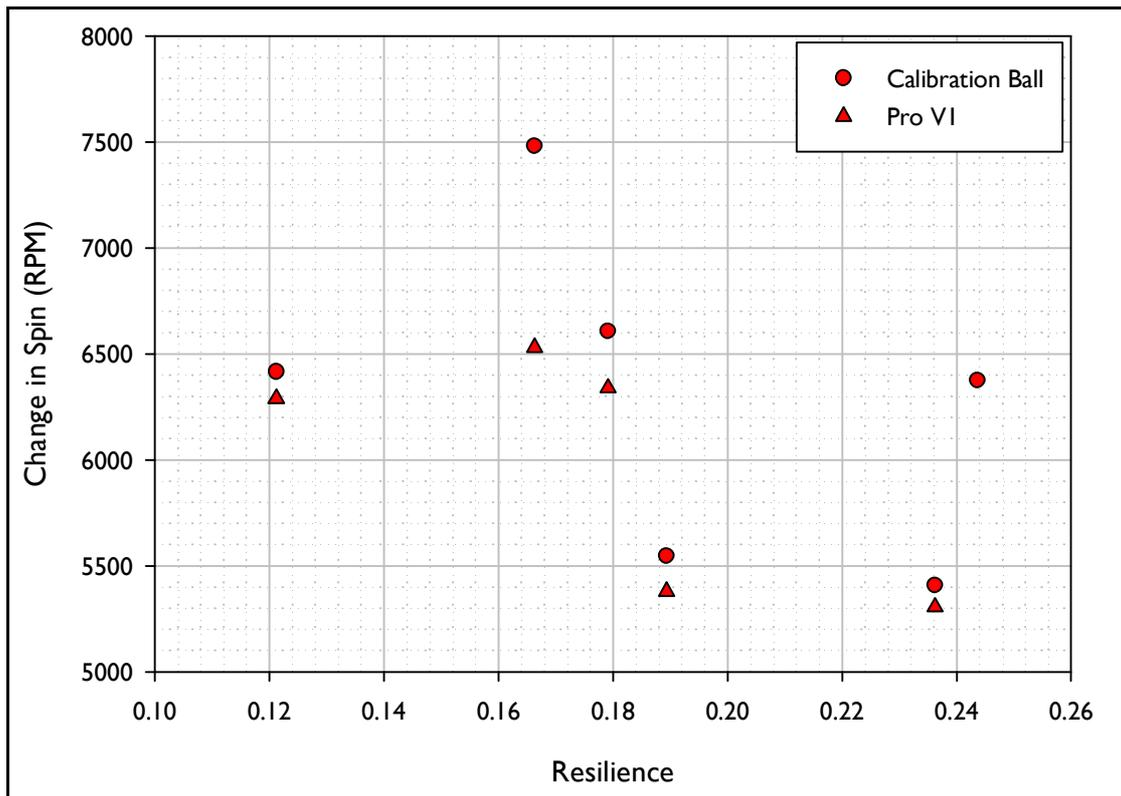
Figure 28. Change in Spin vs. Resilience for the shots fired using the inbound conditions akin to those for a 5 Iron.
