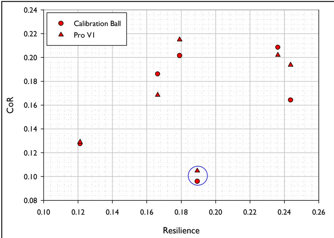
Figure 44. Vertical Coefficient of Restitution (CoR) vs. Resilience for the shots fired using the inbound conditions akin to those for a sand wedge.
