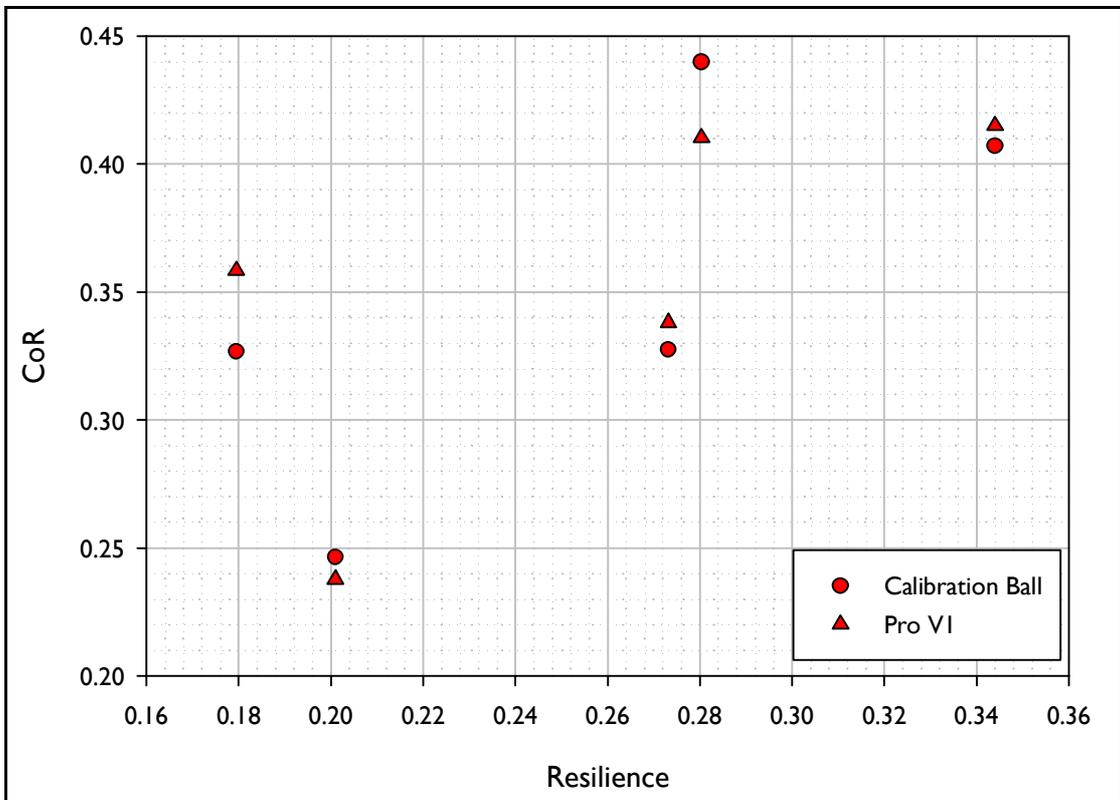
Figure 20. Vertical Coefficient of Restitution (CoR) vs. Resilience for the shots fired using the inbound conditions akin to those for a Driver.
