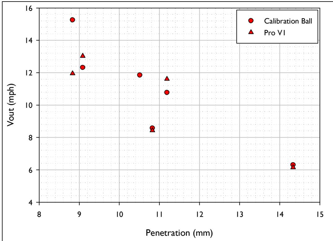
Figure D.1. Outbound speed (Vout) vs. Penetration for the shots fired using the inbound conditions akin to those for a 5 Iron.
