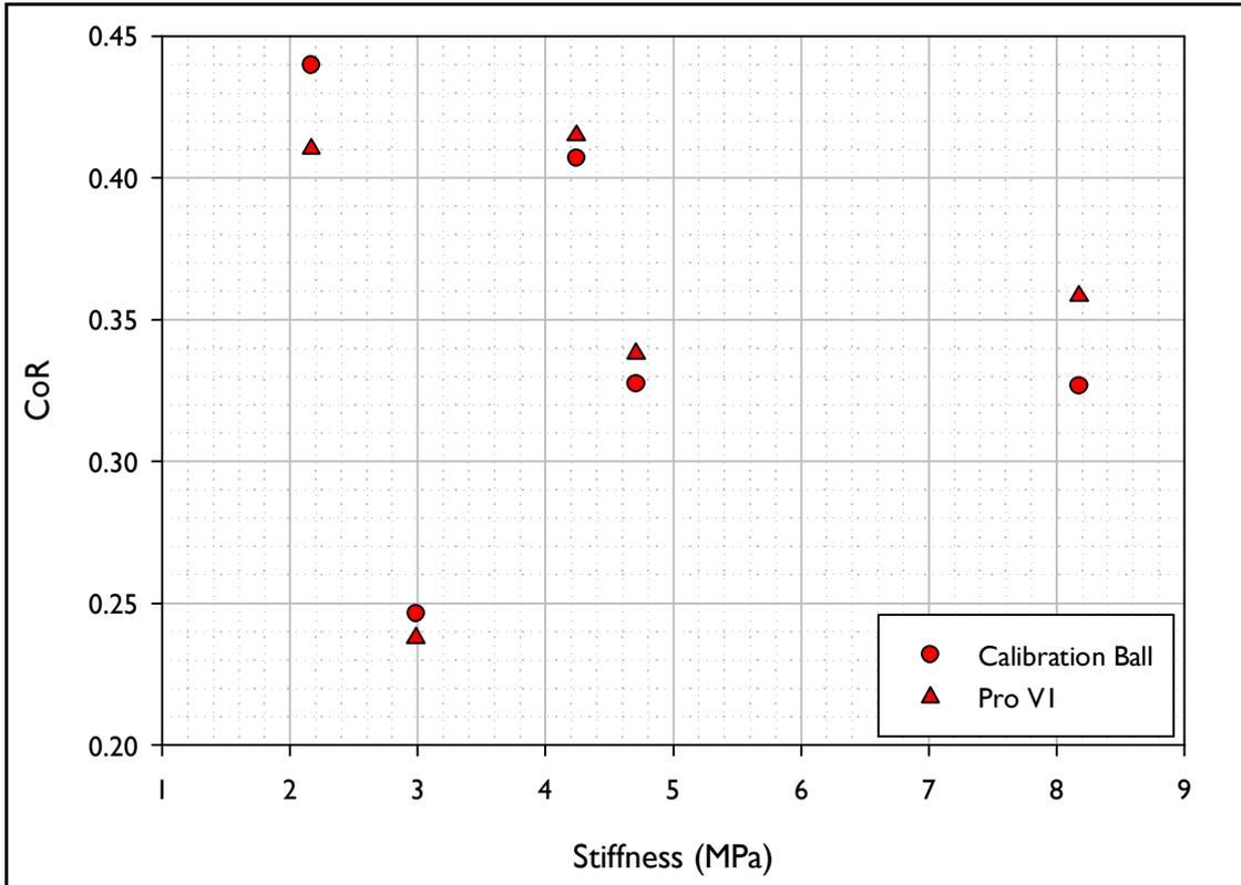
Figure 19. Vertical Coefficient of Restitution (CoR) vs. Stiffness for the shots fired using the inbound conditions akin to those for a Driver.
