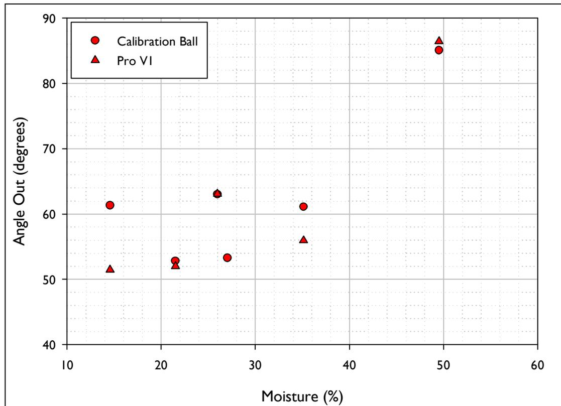
Figure F.2. Outbound Angle after Impact vs. Moisture for the shots fired using the inbound conditions akin to those for a 5 Iron.
