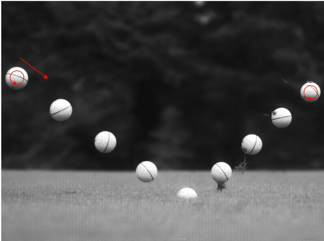
Figure 9. A composite image comprising selected frames from a typical driver impact.
