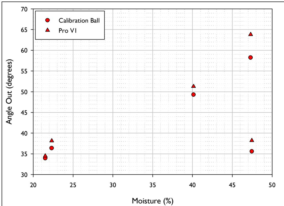
Figure C.2. Outbound Angle after Impact vs. Moisture for the shots fired using the inbound conditions akin to those for a Driver.
