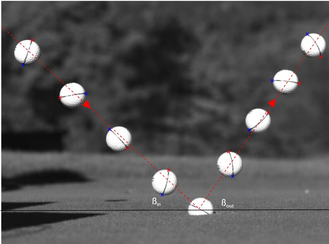
Figure 2. A composite of 9 frames from a recorded video illustrating typical field of view and also how pre- and post- speed, spin and angle can be calculated.
