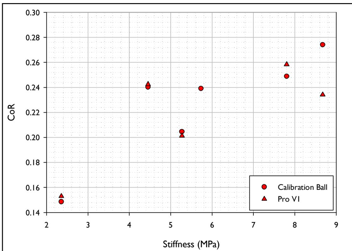
Figure 31. Vertical Coefficient of Restitution (CoR) vs. Stiffness for the shots fired using the inbound conditions akin to those for a 5 Iron.
