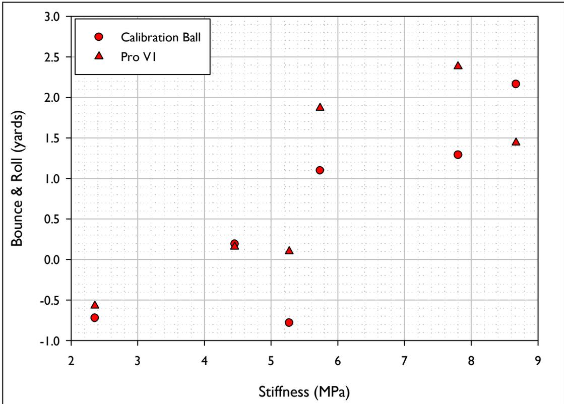
Figure 41. Bounce & Roll vs. Stiffness for the shots fired using the inbound conditions akin to those for a sand wedge.
