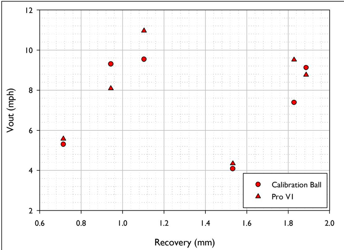
Figure H.1. Outbound speed (Vout) vs. Recovery for the shots fired using the inbound conditions akin to those for a Sand Wedge.
