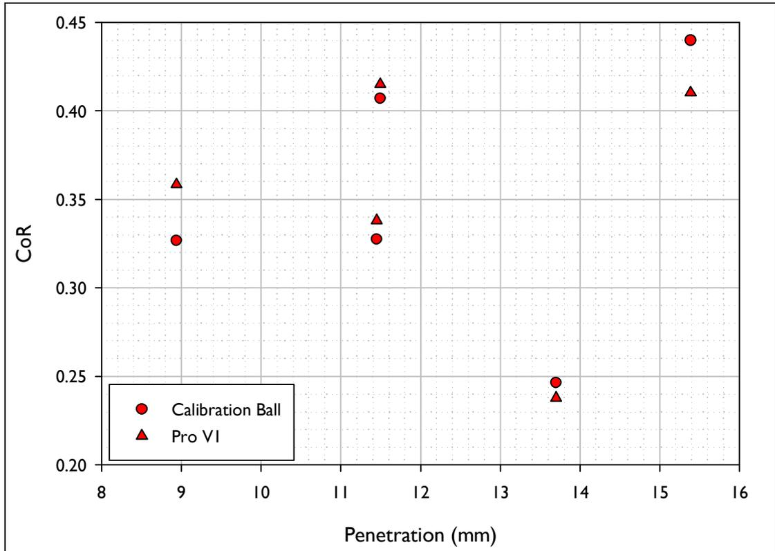
Figure A.5. Vertical Coefficient of Restitution (CoR) vs. Penetration for the shots fired using the inbound conditions akin to those for a Driver.
