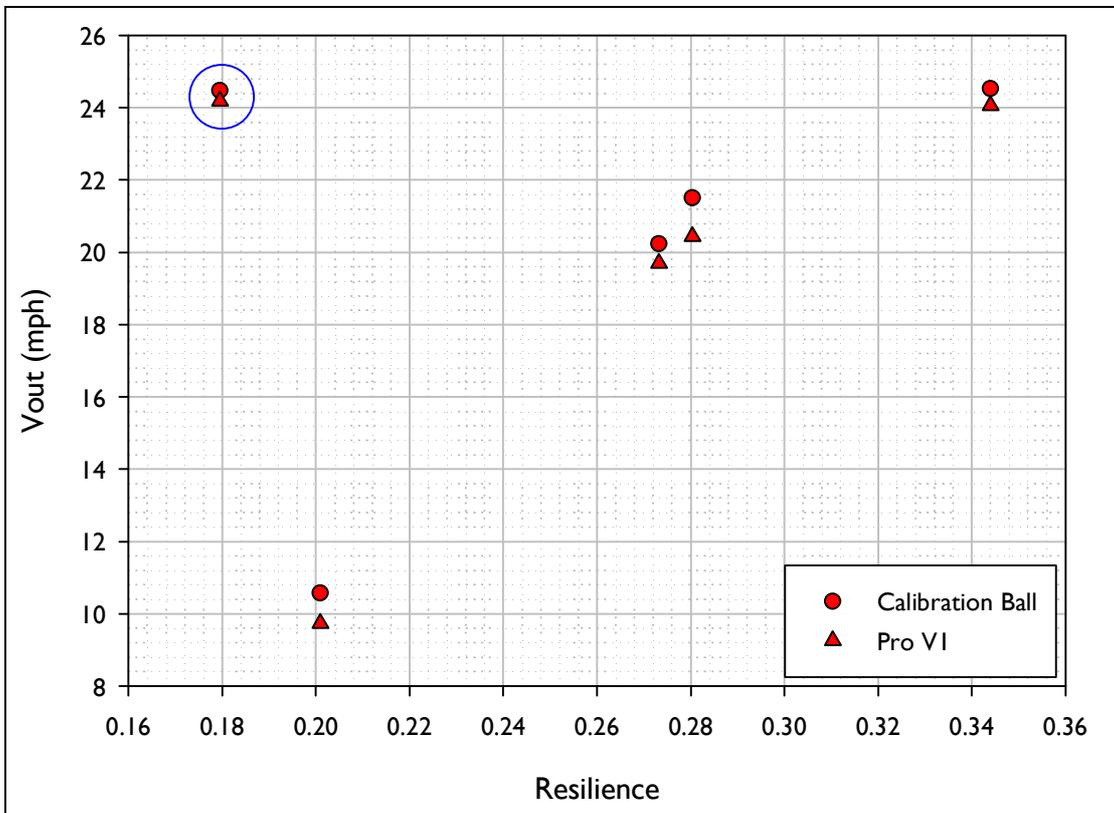
Figure 12. Outbound speed (Vout) vs. Resilience for the shots fired using the inbound conditions akin to those for a Driver.
