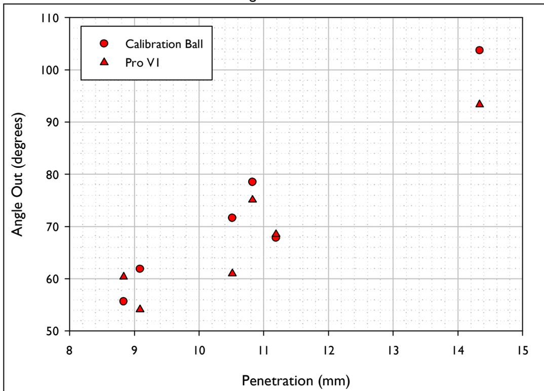
Figure G.2. Outbound Angle after Impact vs. Penetration for the shots fired using the inbound conditions akin to those for a Sand Wedge.
