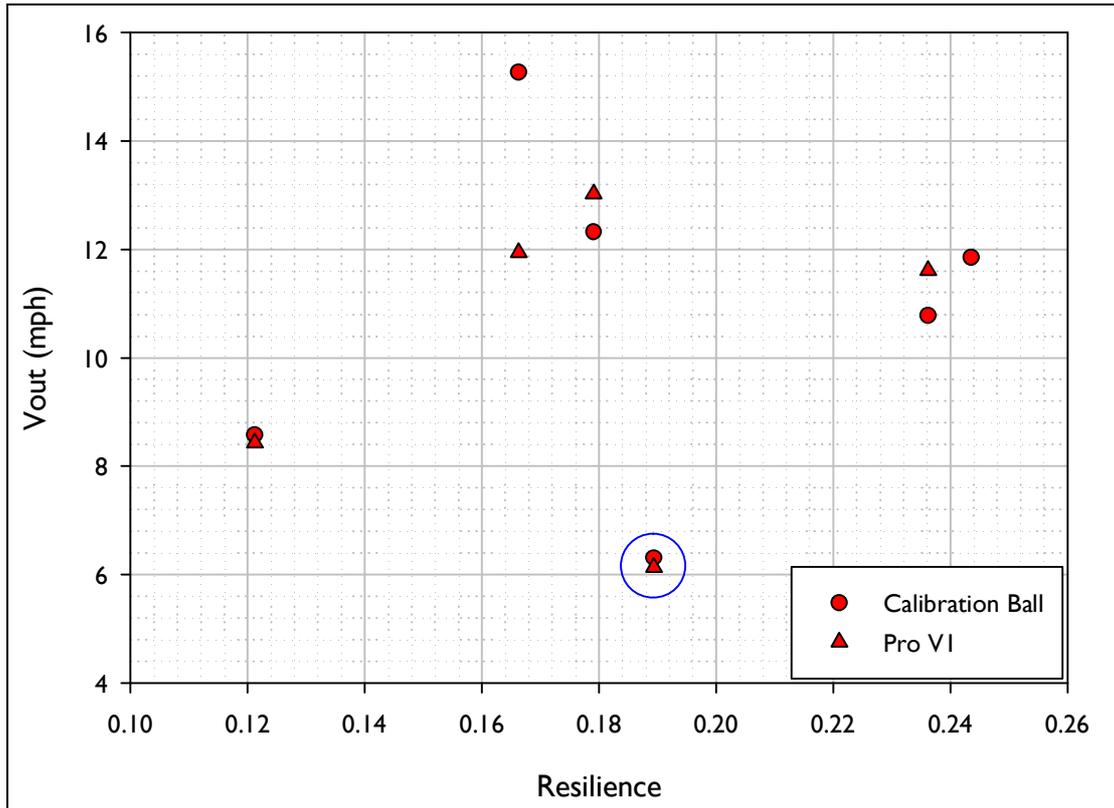
Figure 24. Outbound speed (Vout) vs. Resilience for the shots fired using the inbound conditions akin to those for a 5 Iron.
