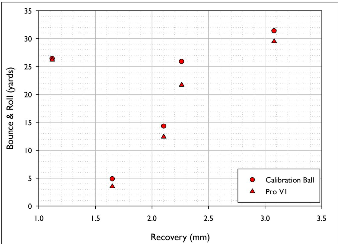
Figure B.4. Bounce & Roll vs. Recovery for the shots fired using the inbound conditions akin to those for a Driver.
