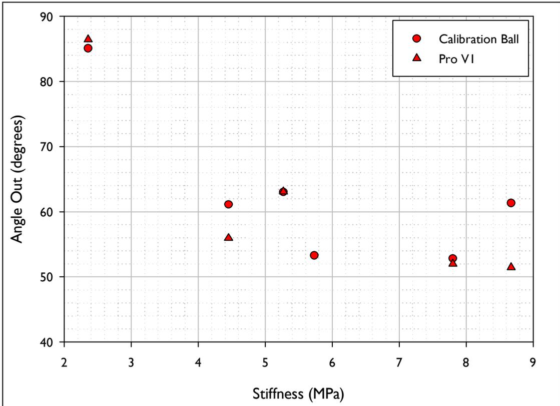
Figure 25. Outbound Angle after Impact vs. Stiffness for the shots fired using the inbound conditions akin to those for a 5 Iron.
