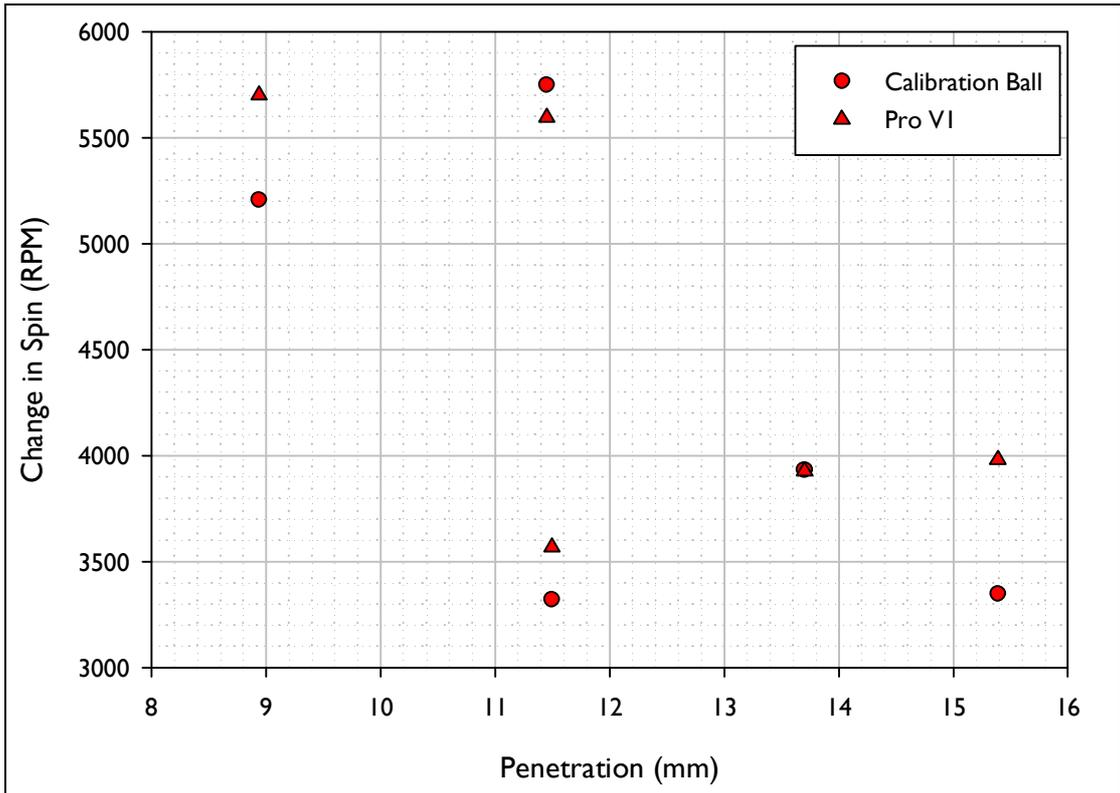
Figure A.3. Change in Spin vs. Penetration for the shots fired using the inbound conditions akin to those for a Driver.
