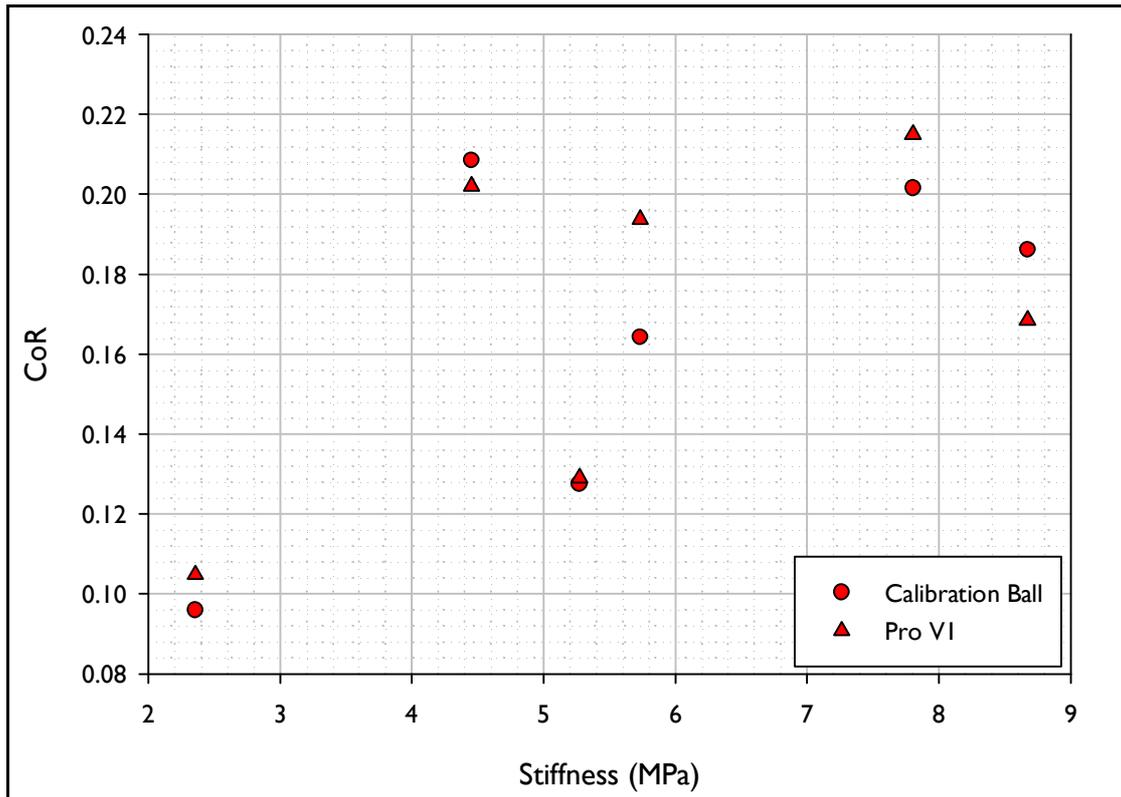
Figure 43. Vertical Coefficient of Restitution (CoR) vs. Stiffness for the shots fired using the inbound conditions akin to those for a sand wedge.
