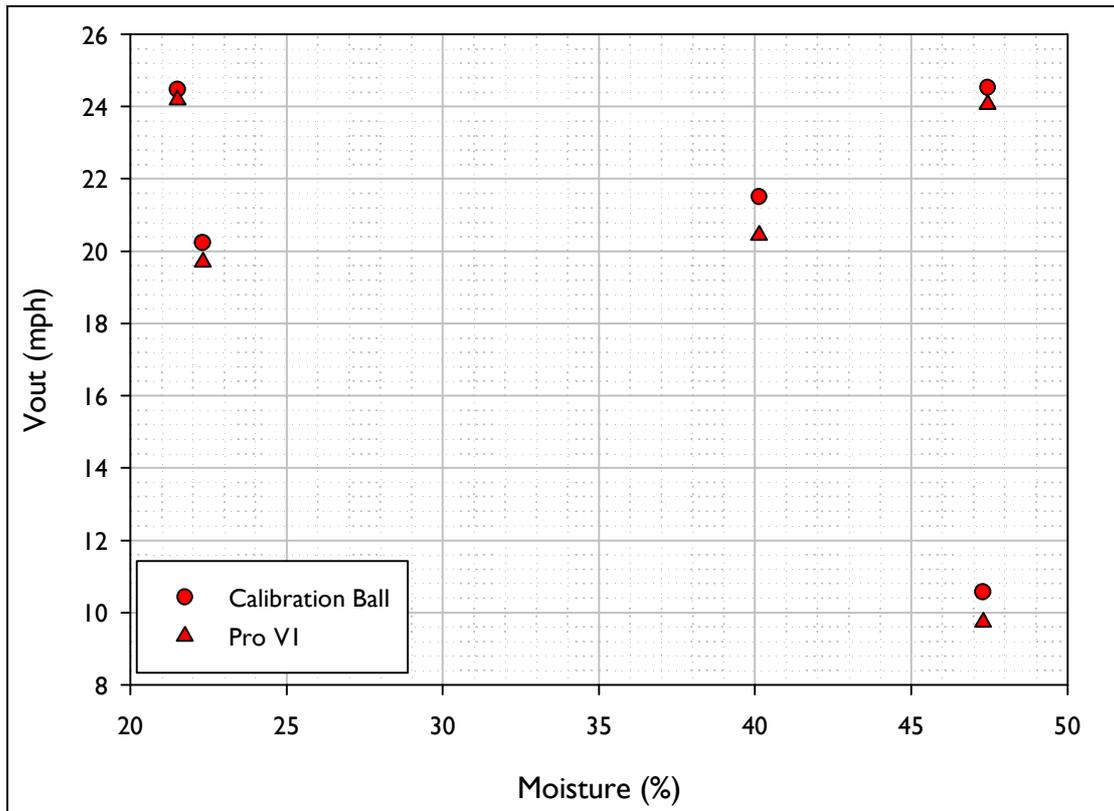
Figure C.1. Outbound speed (Vout) vs. Moisture for the shots fired using the inbound conditions akin to those for a Driver.
