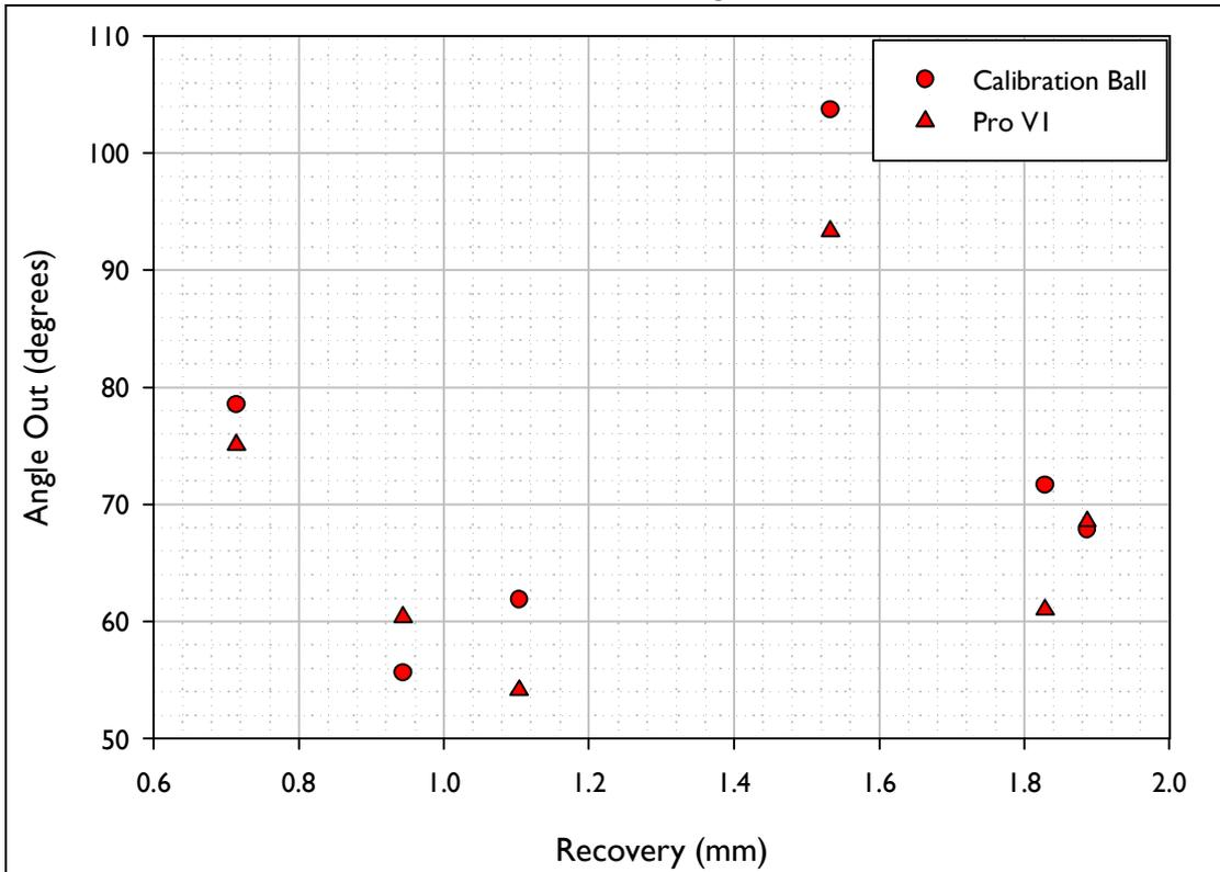
Figure H.2. Outbound Angle after Impact vs. Recovery for the shots fired using the inbound conditions akin to those for a Sand Wedge.
