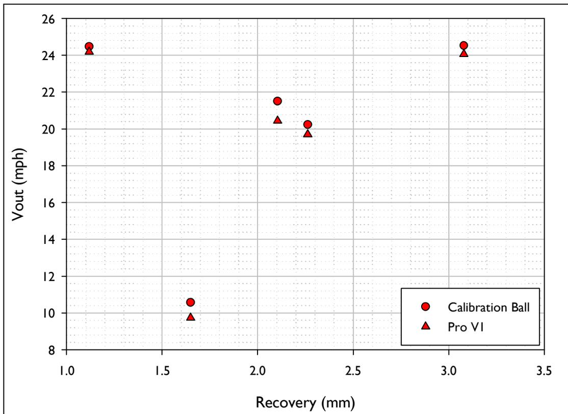
Figure B.1. Outbound speed (Vout) vs. Recovery for the shots fired using the inbound conditions akin to those for a Driver.
