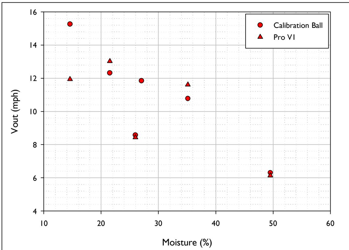
Figure F.1. Outbound speed ( $V_{out}$ ) vs. Moisture for the shots fired using the inbound conditions akin to those for a 5 Iron.
