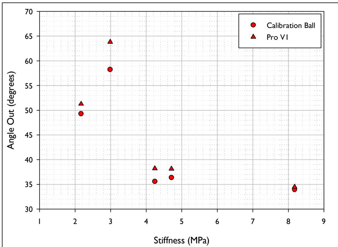
Figure 13. Outbound Angle after Impact vs. Stiffness for the shots fired using the inbound conditions akin to those for a Driver.
