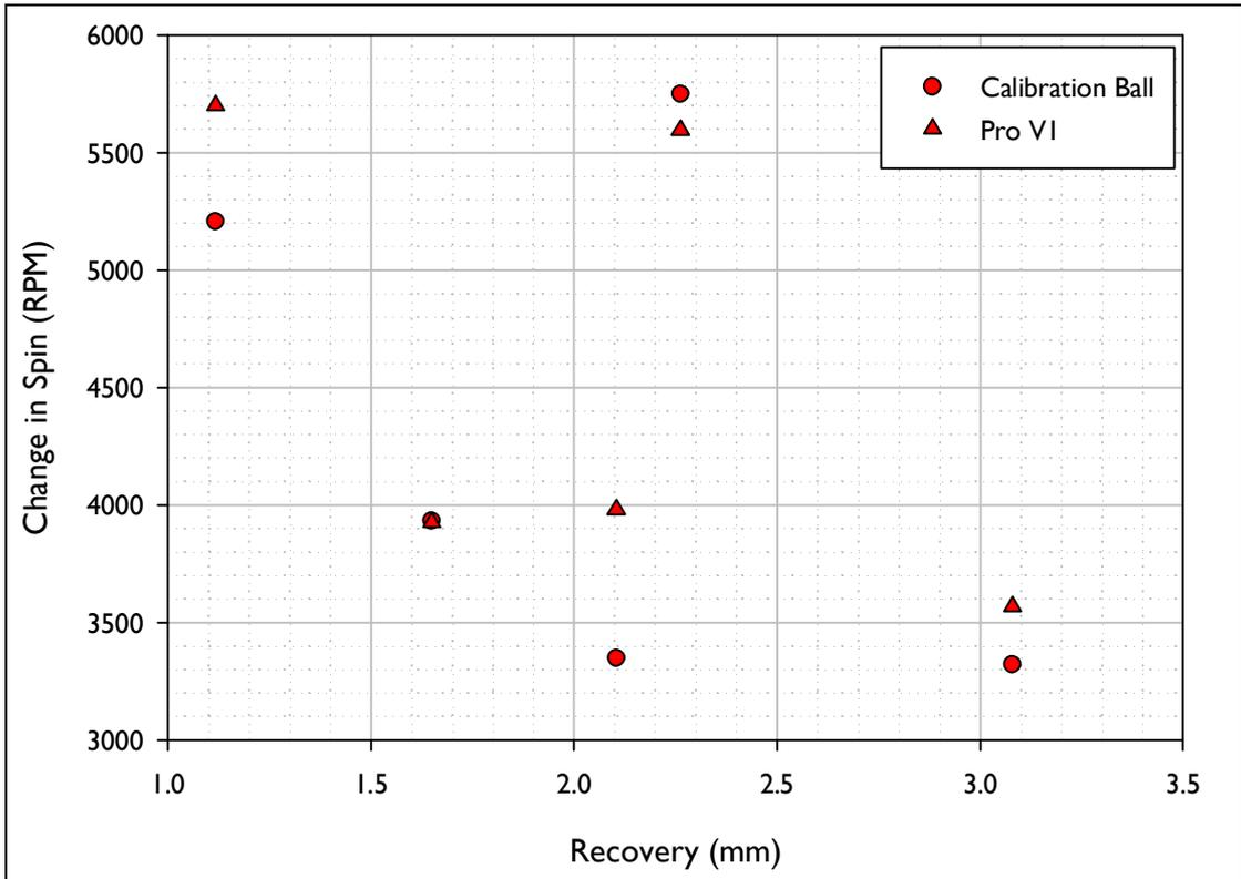
Figure B.3. Change in Spin vs. Recovery for the shots fired using the inbound conditions akin to those for a Driver.
