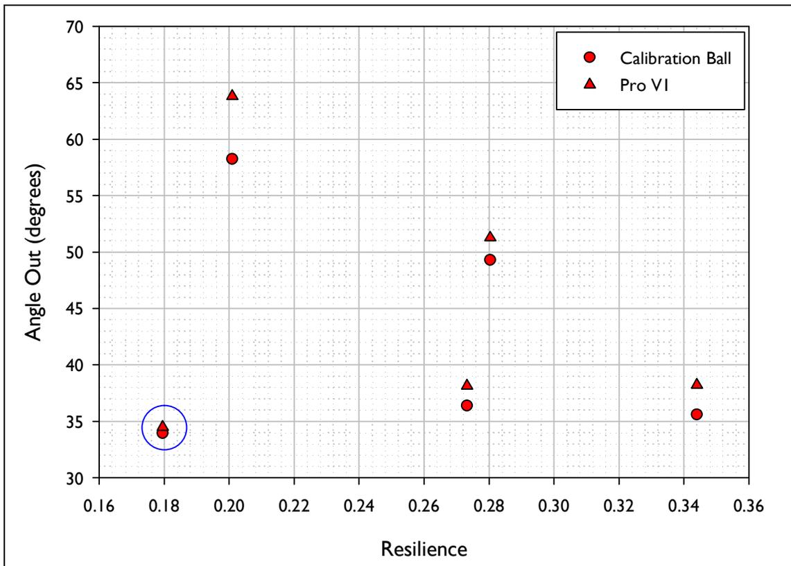
Figure 14. Outbound Angle after Impact vs. Resilience for the shots fired using the inbound conditions akin to those for a Driver.
