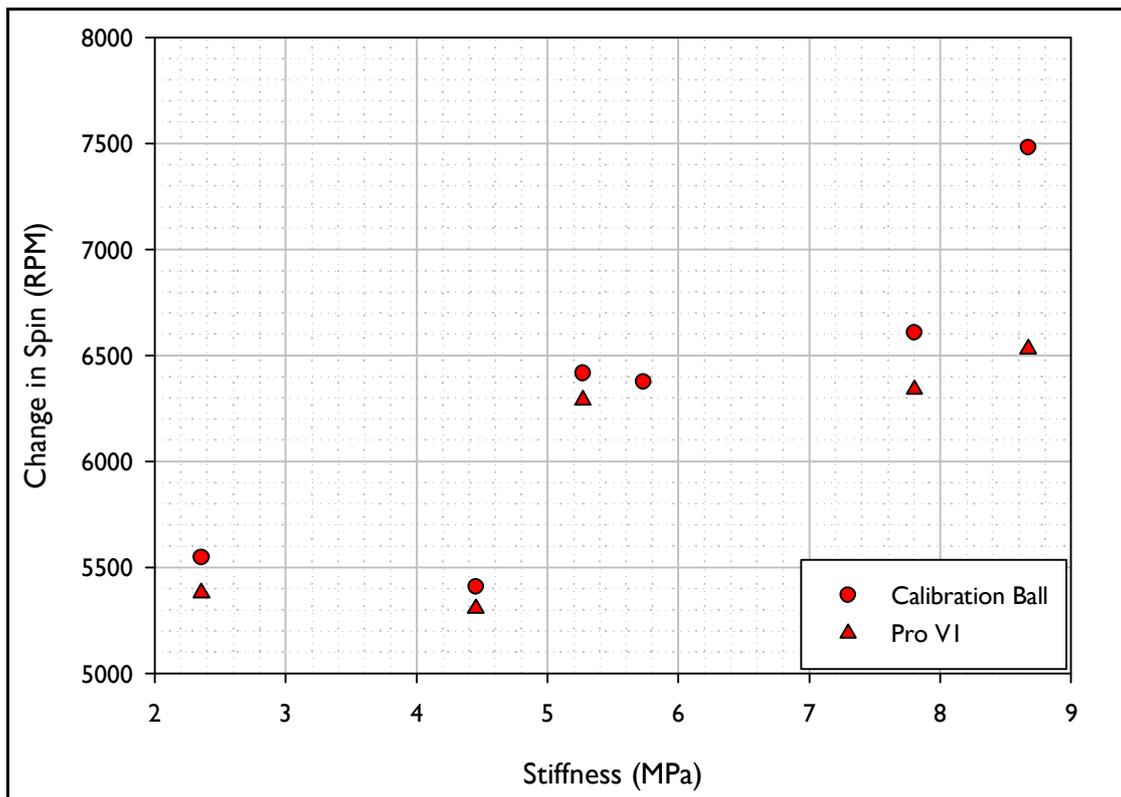
Figure 27. Change in Spin vs. Stiffness for the shots fired using the inbound conditions akin to those for a 5 Iron.
