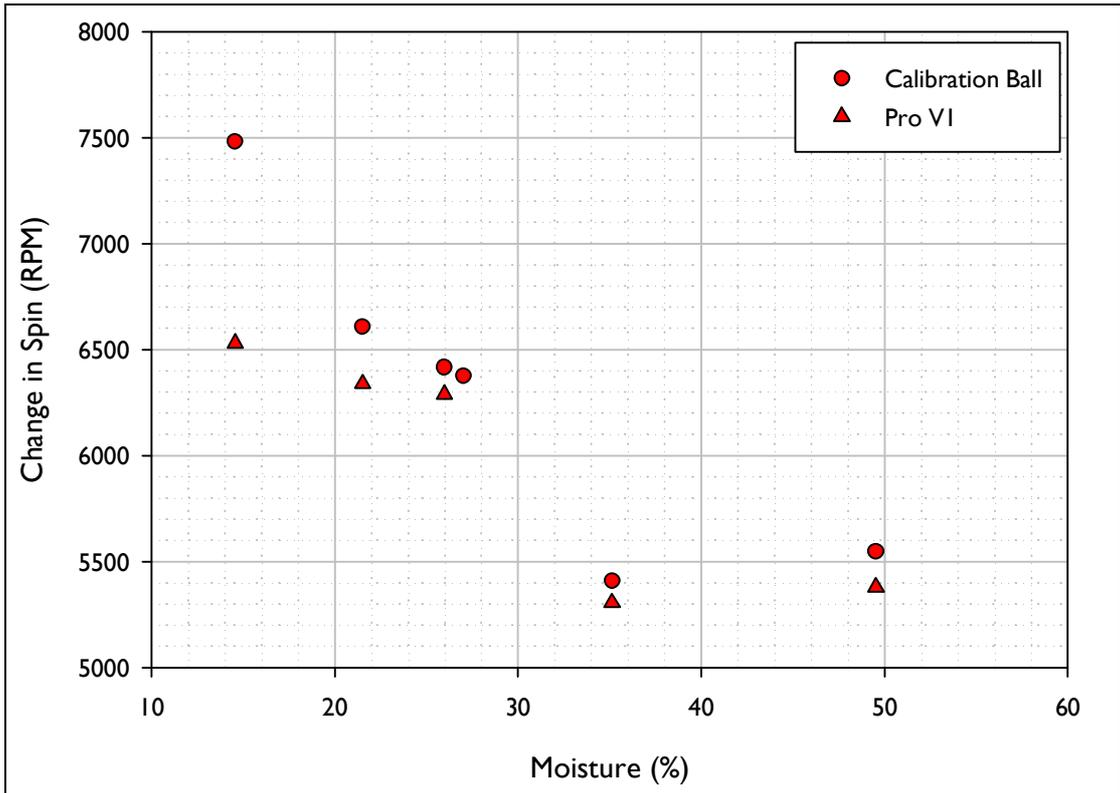
Figure F.3. Change in Spin vs. Moisture for the shots fired using the inbound conditions akin to those for a 5 Iron.
