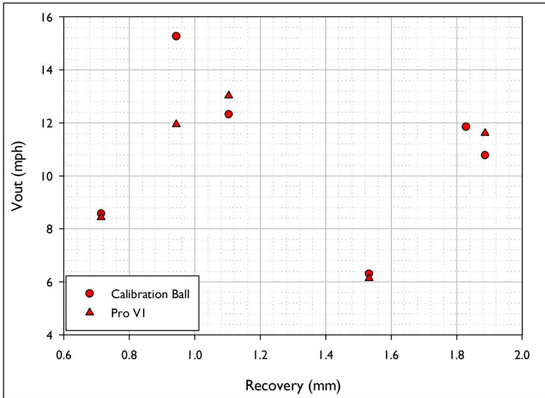
Figure E.1. Outbound speed (Vout) vs. Recovery for the shots fired using the inbound conditions akin to those for a 5 Iron.
