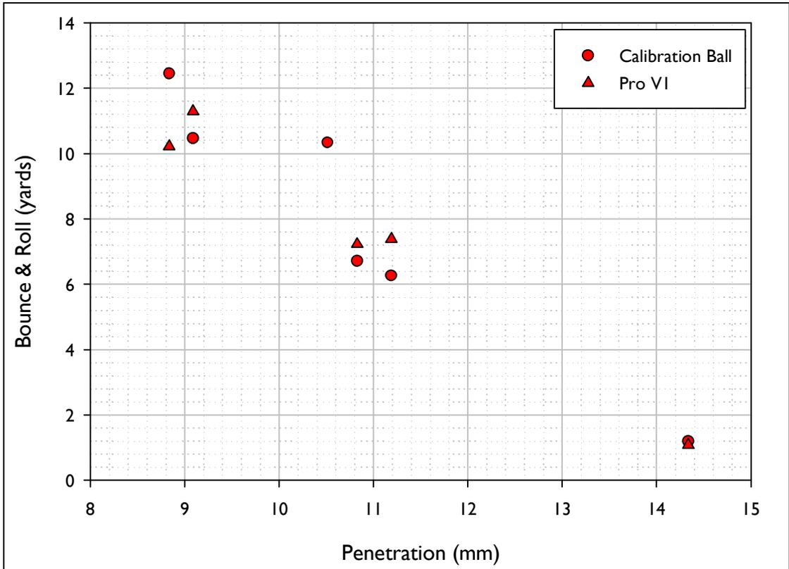
Figure D.4. Bounce & Roll vs. Penetration for the shots fired using the inbound conditions akin to those for a 5 Iron.
