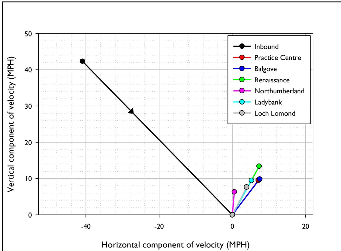
Figure 22. Inbound and Outbound velocity vectors for the Calibration ball when launched with 5 iron impact conditions.
