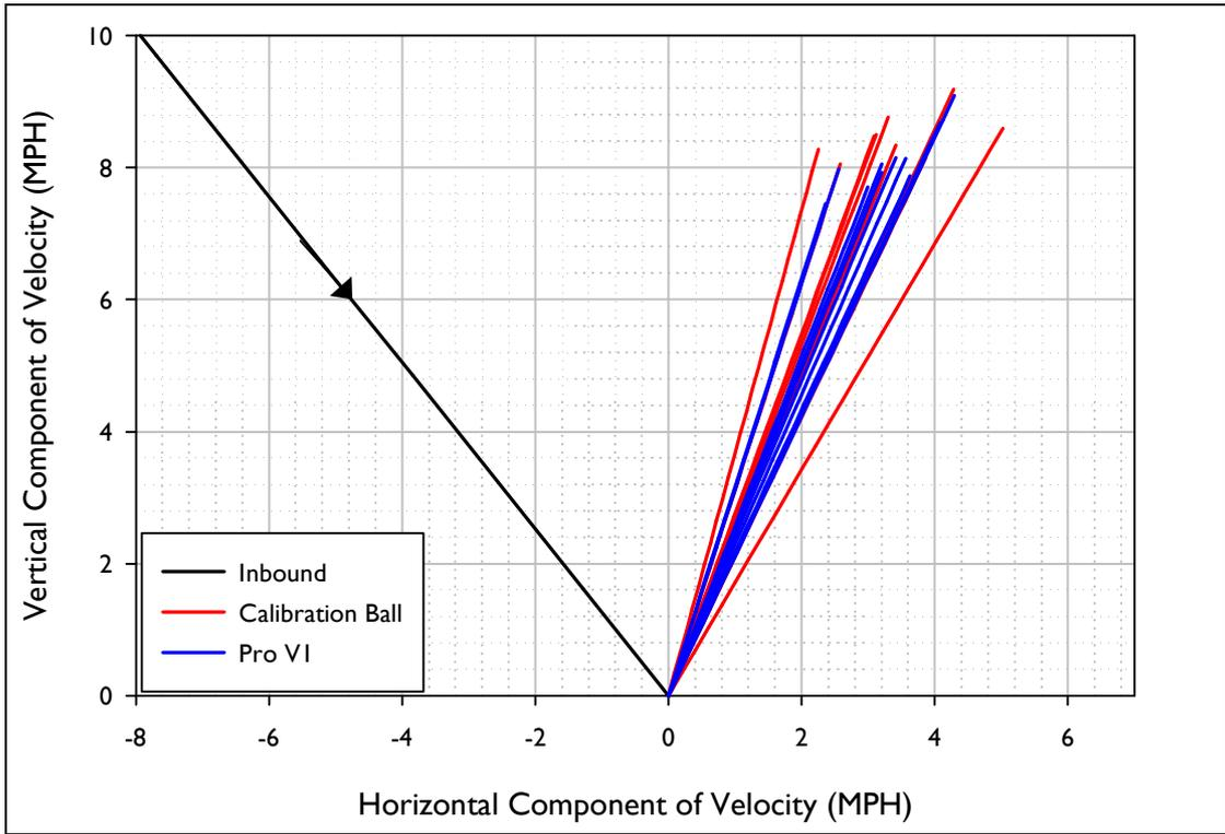
Figure 7. Outbound velocity vectors for the individual sand wedge shots at Ladybank
