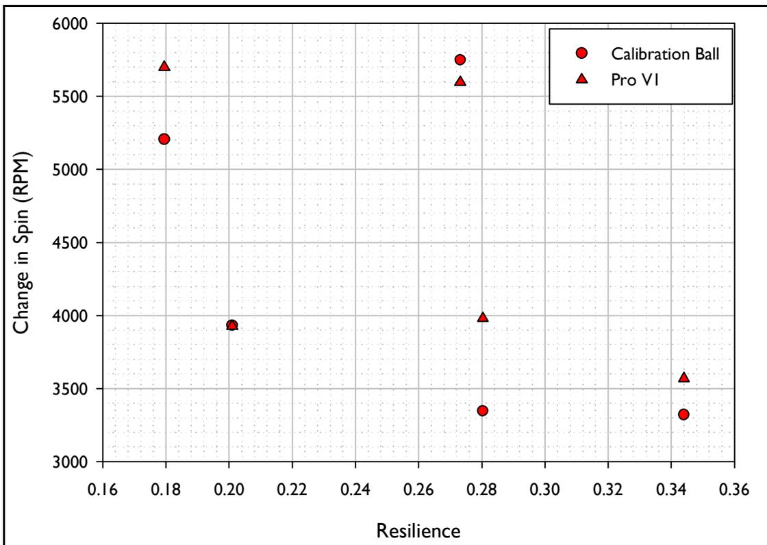
Figure 16. Change in Spin vs. Resilience for the shots fired using the inbound conditions akin to those for a Driver.
