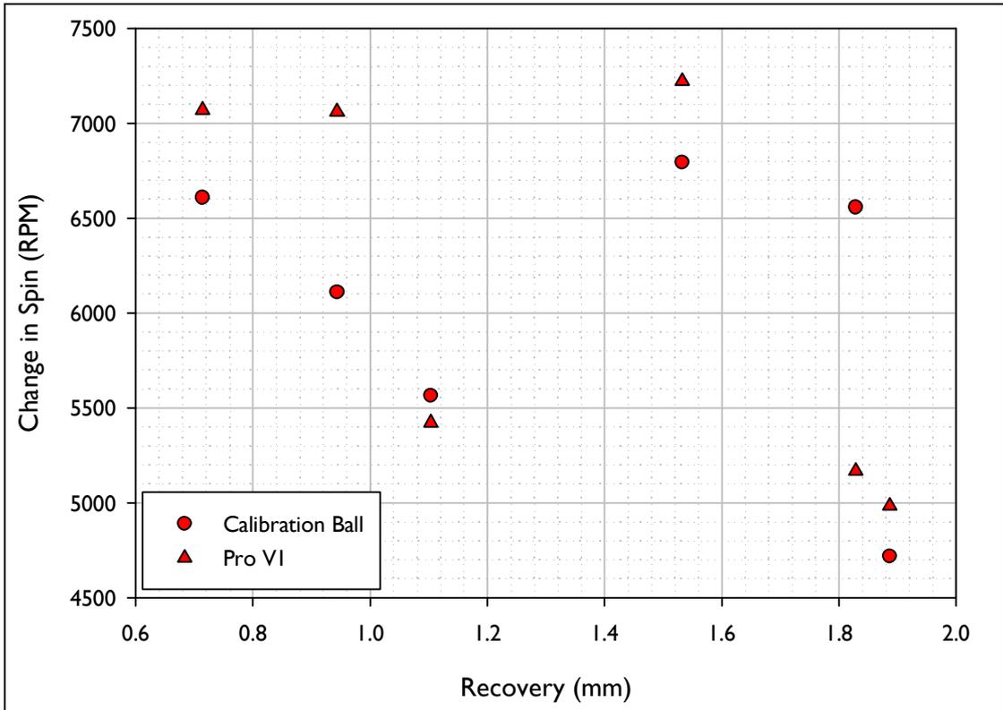
Figure H.3. Change in Spin vs. Recovery for the shots fired using the inbound conditions akin to those for a Sand Wedge.
