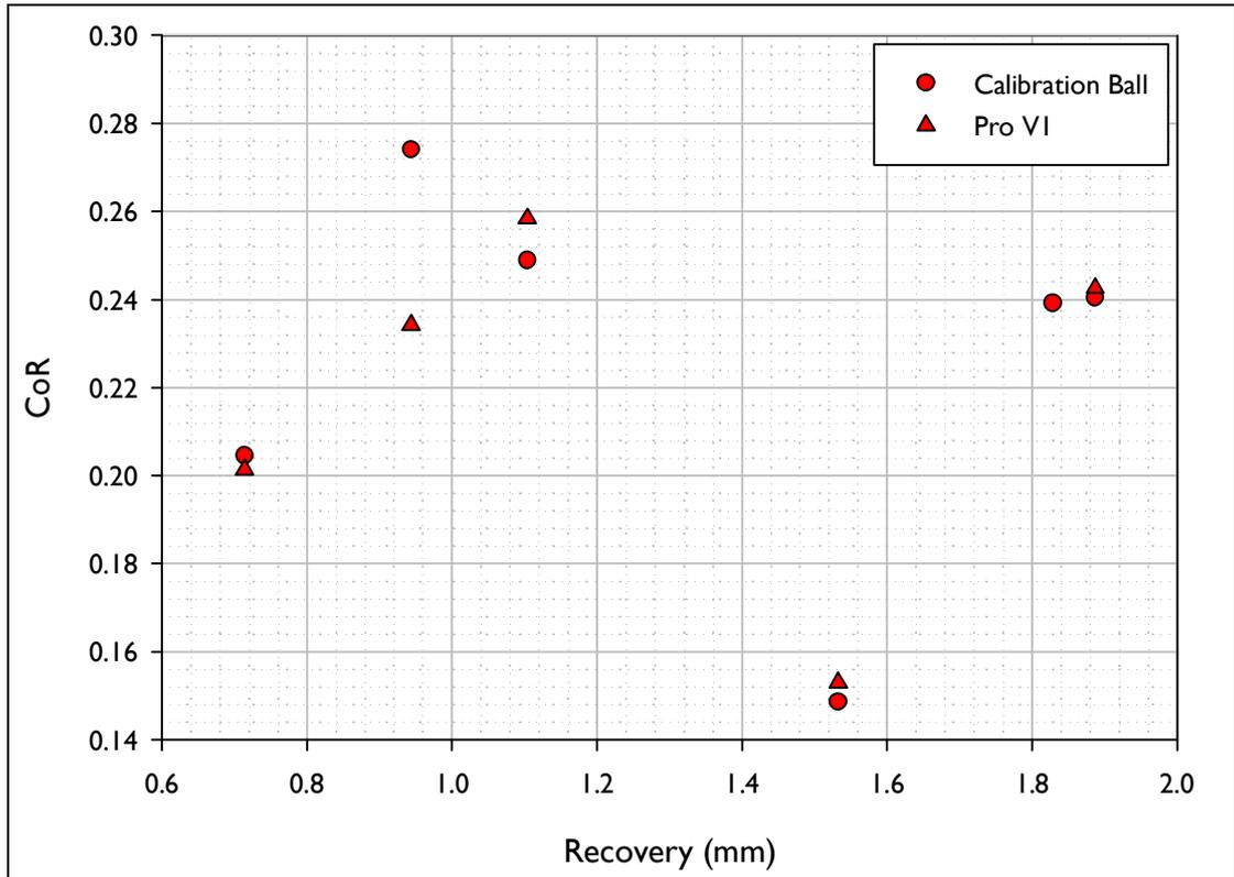
Figure E.5. Vertical Coefficient of Restitution (CoR) vs. Recovery for the shots fired using the inbound conditions akin to those for a 5 Iron.
