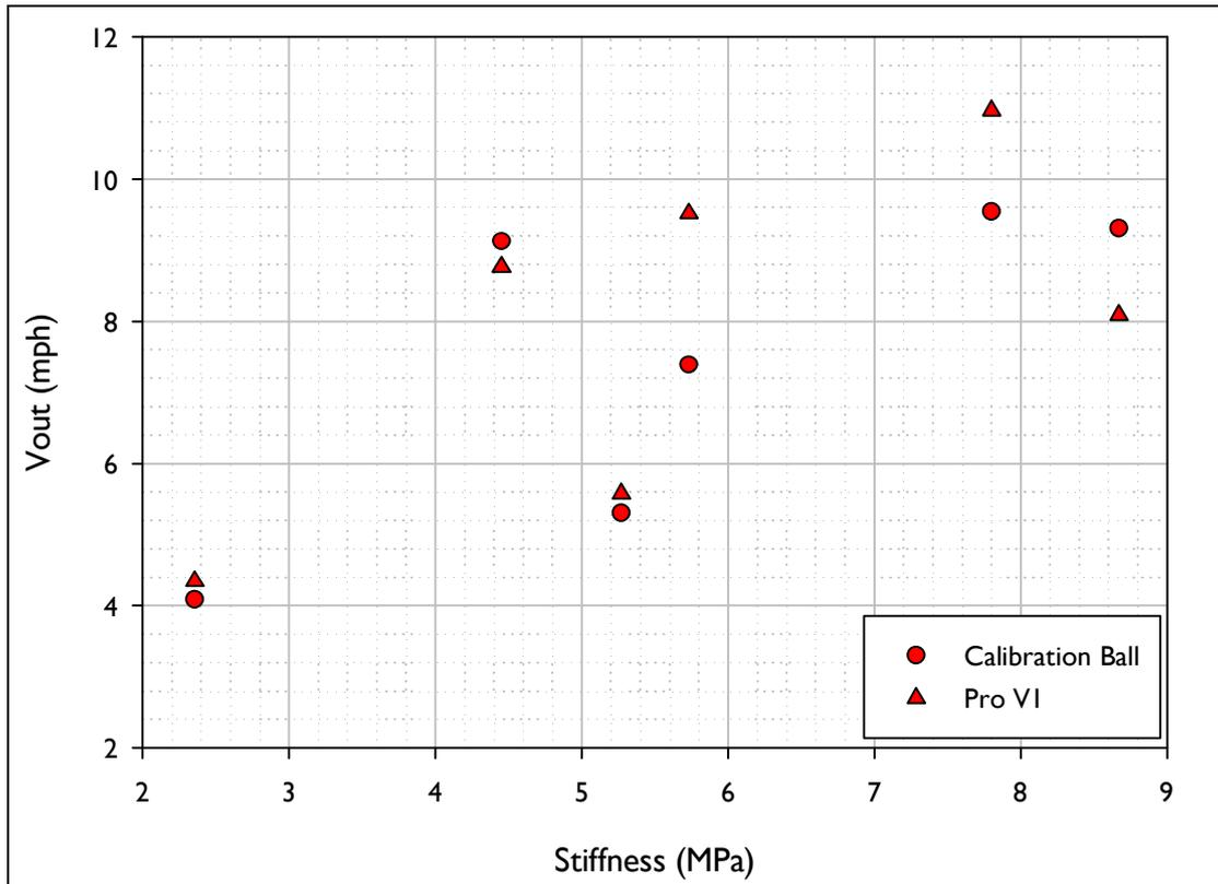
Figure 35. Outbound speed (Vout) vs. Stiffness for the shots fired using the inbound conditions akin to those for a sand wedge.
