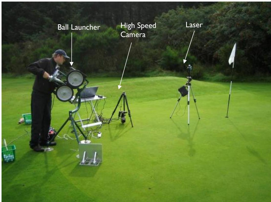
Figure 3. The testing set up comprising the modified pitching machine, high speed camera and distance measuring laser equipment.
