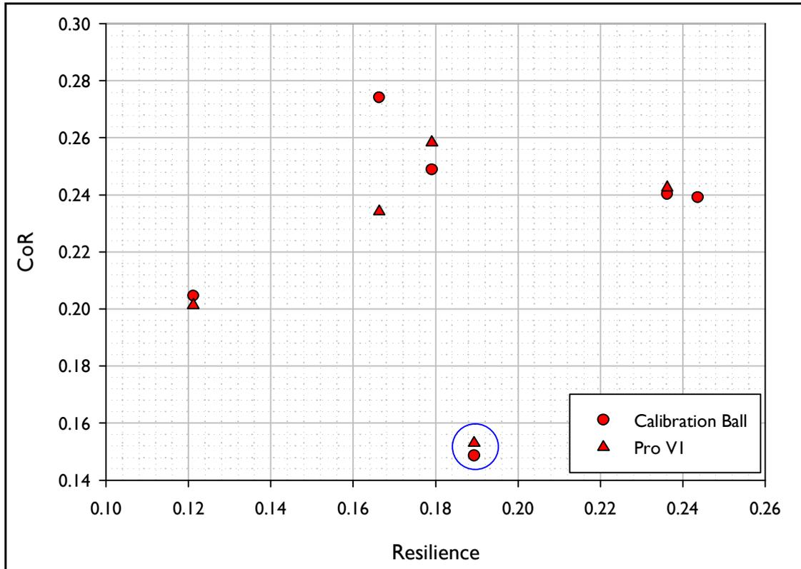
Figure 32. Vertical Coefficient of Restitution (CoR) vs. Resilience for the shots fired using the inbound conditions akin to those for a 5 Iron.
