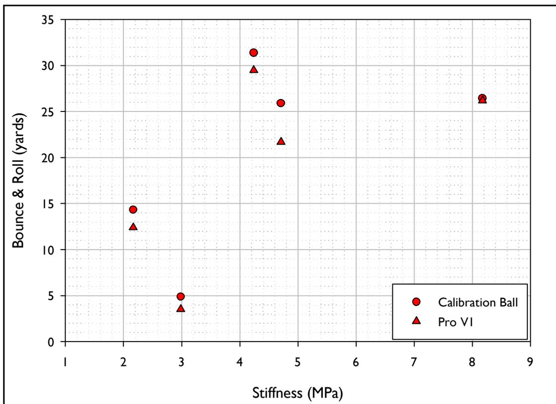
Figure 17. Bounce & Roll vs. Stiffness for the shots fired using the inbound conditions akin to those for a Driver.
