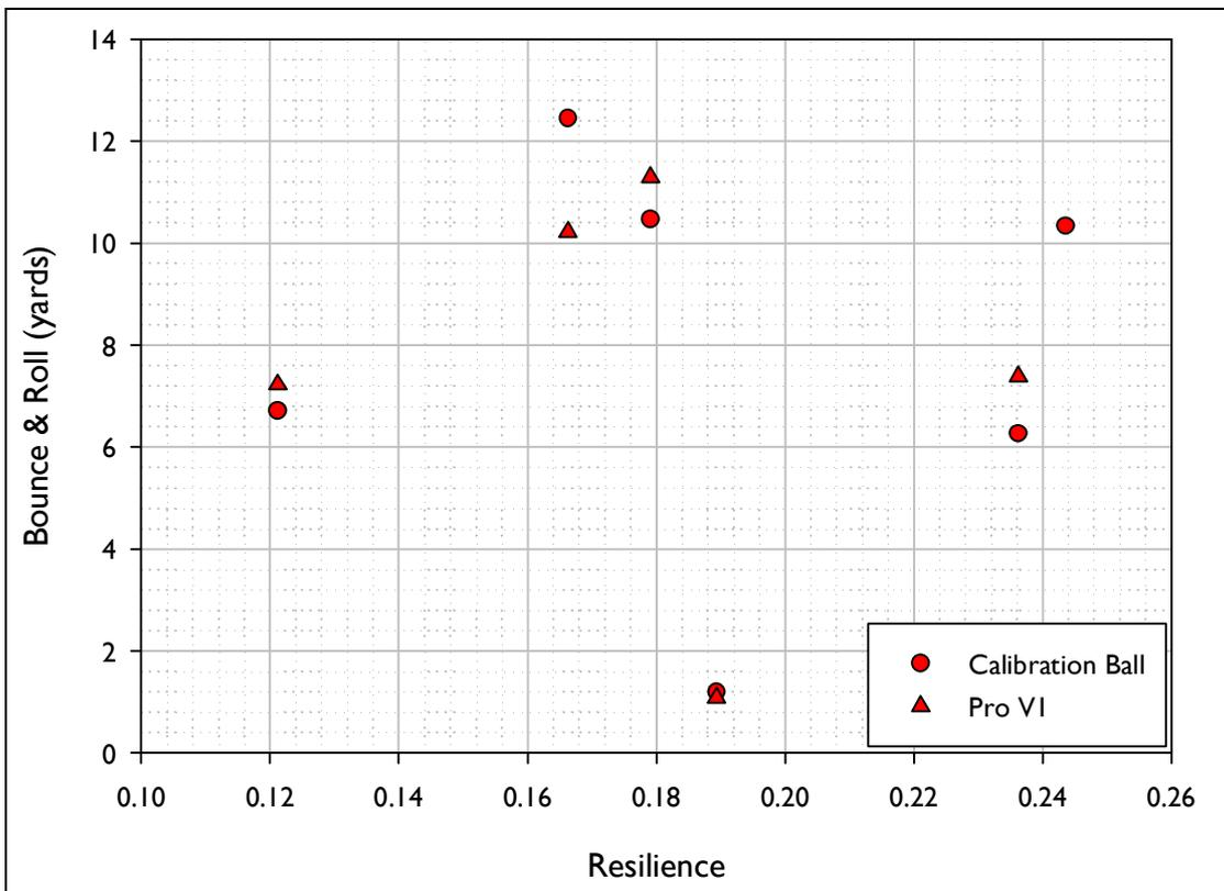
Figure 30. Bounce & Roll vs. Resilience for the shots fired using the inbound conditions akin to those for a sand wedge.
