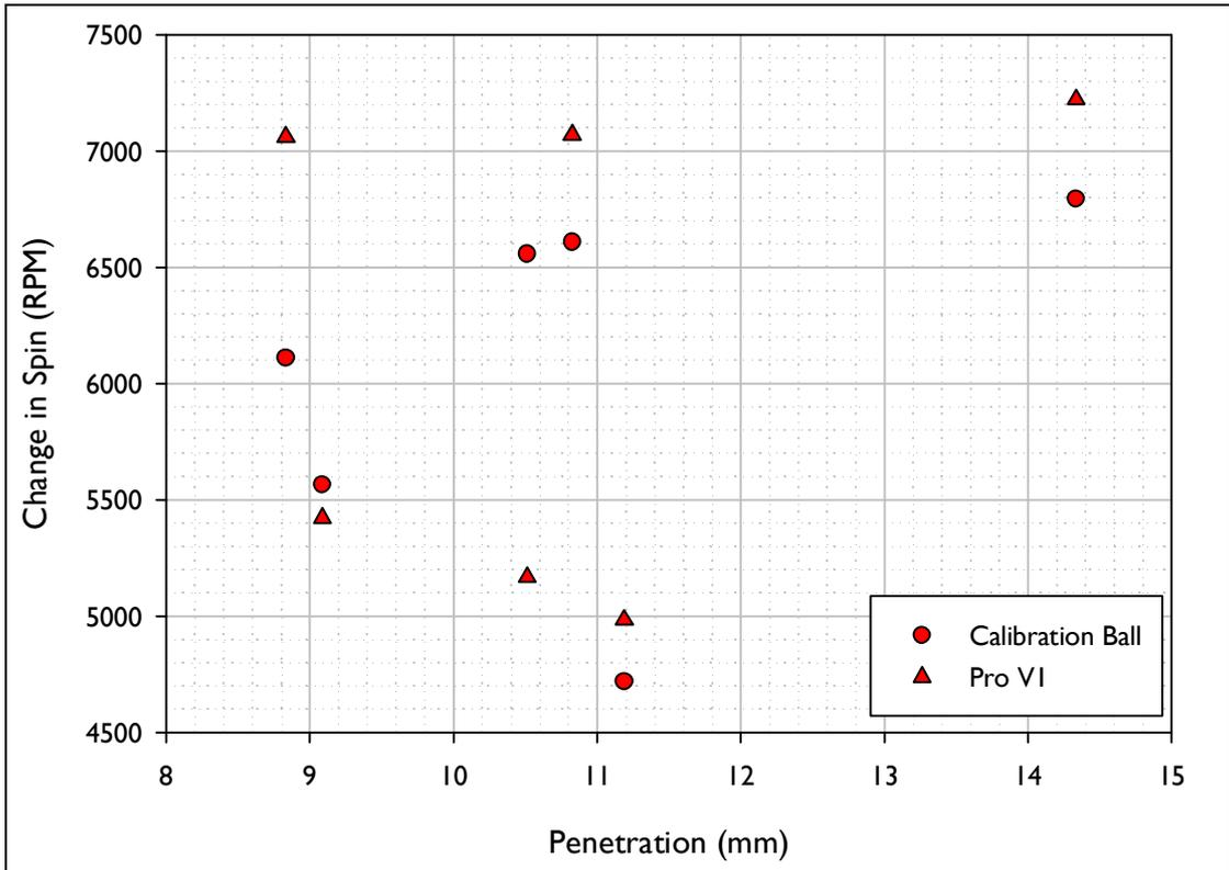
Figure G.3. Change in Spin vs. Penetration for the shots fired using the inbound conditions akin to those for a Sand Wedge.
