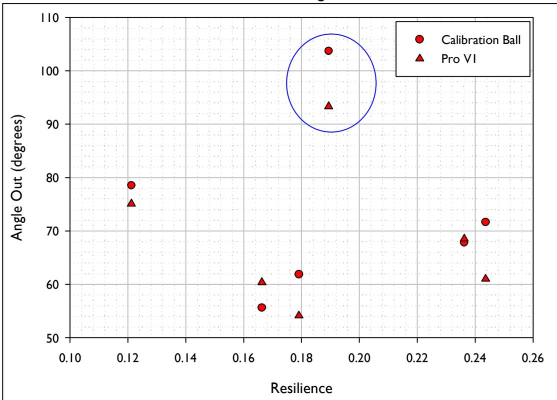
Figure 38. Outbound Angle after Impact vs. Resilience for the shots fired using the inbound conditions akin to those for a sand wedge.
