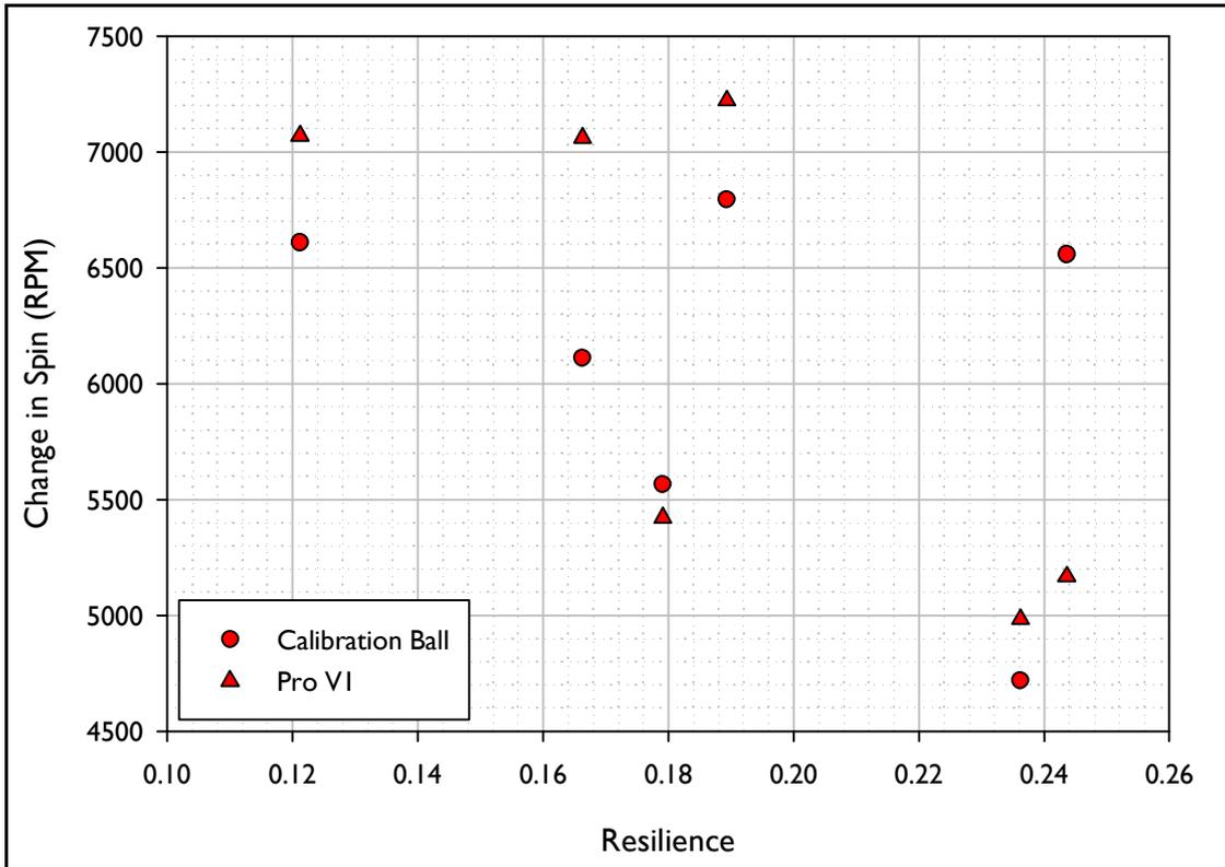
Figure 40. Change in Spin vs. Resilience for the shots fired using the inbound conditions akin to those for a sand wedge.
