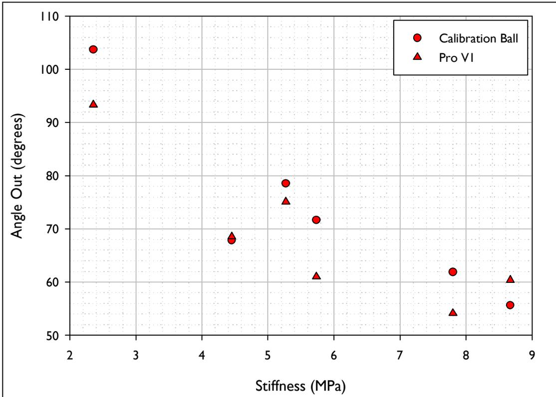
Figure 37. Outbound Angle after Impact vs. Stiffness for the shots fired using the inbound conditions akin to those for a sand wedge.
