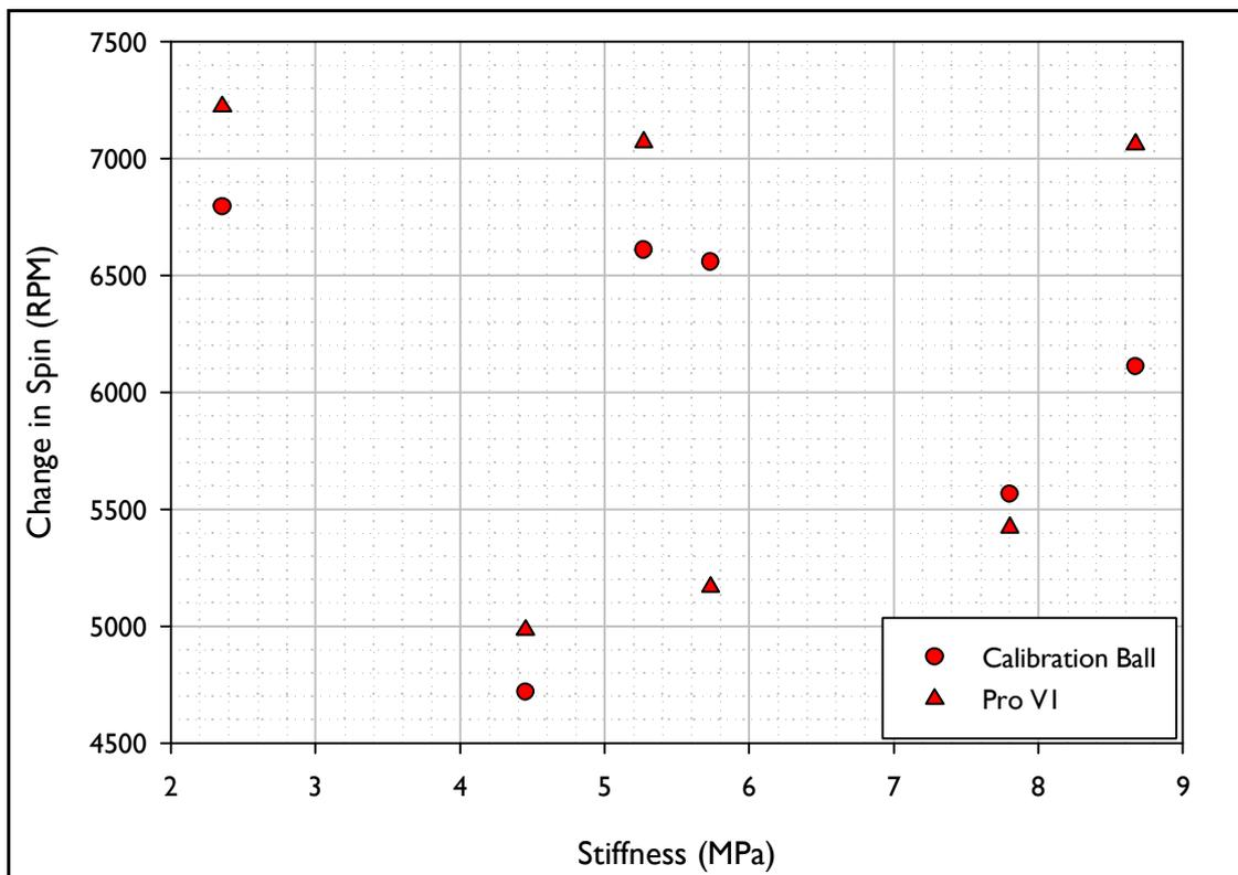
Figure 39. Change in Spin vs. Stiffness for the shots fired using the inbound conditions akin to those for a sand wedge.
