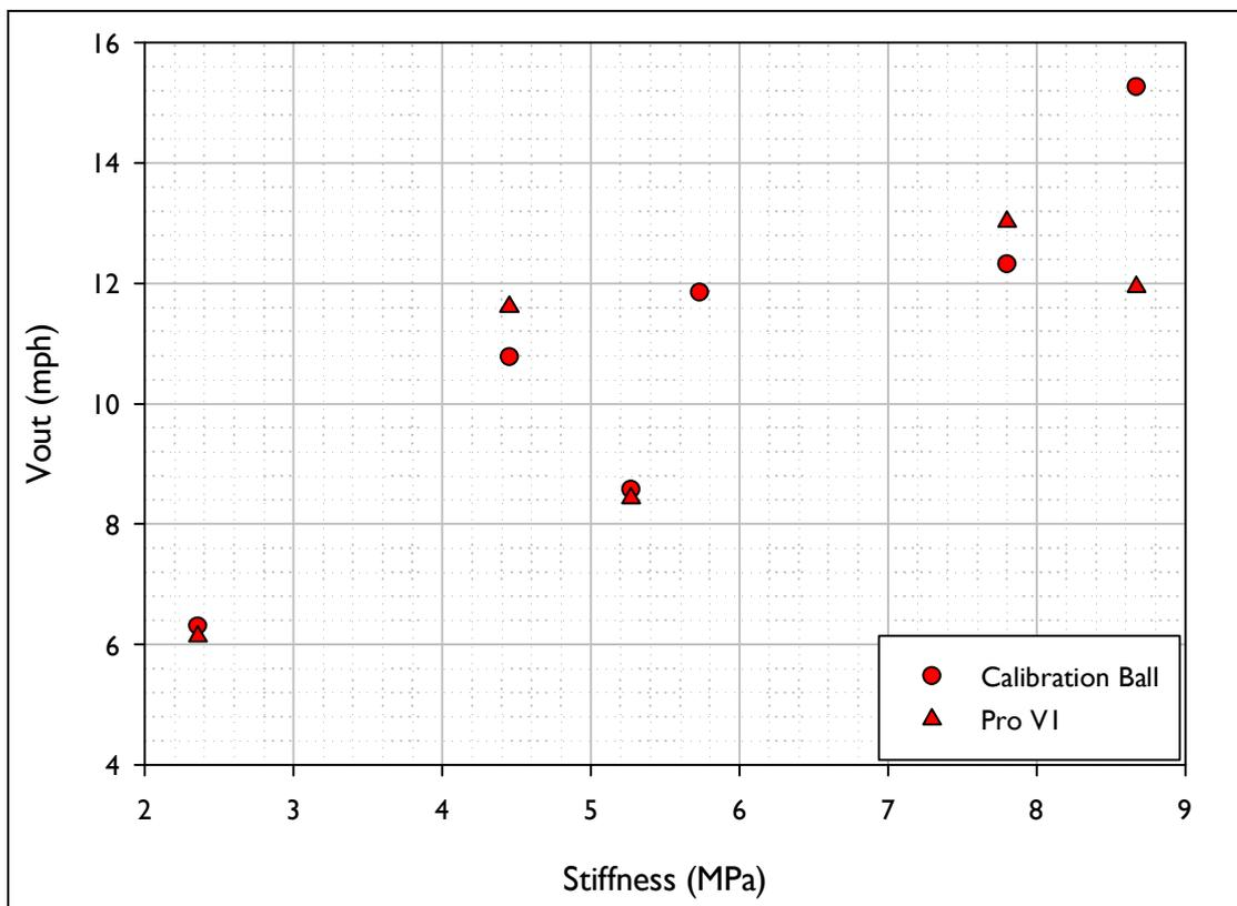
Figure 23. Outbound speed (Vout) vs. Stiffness for the shots fired using the inbound conditions akin to those for a 5 Iron.
