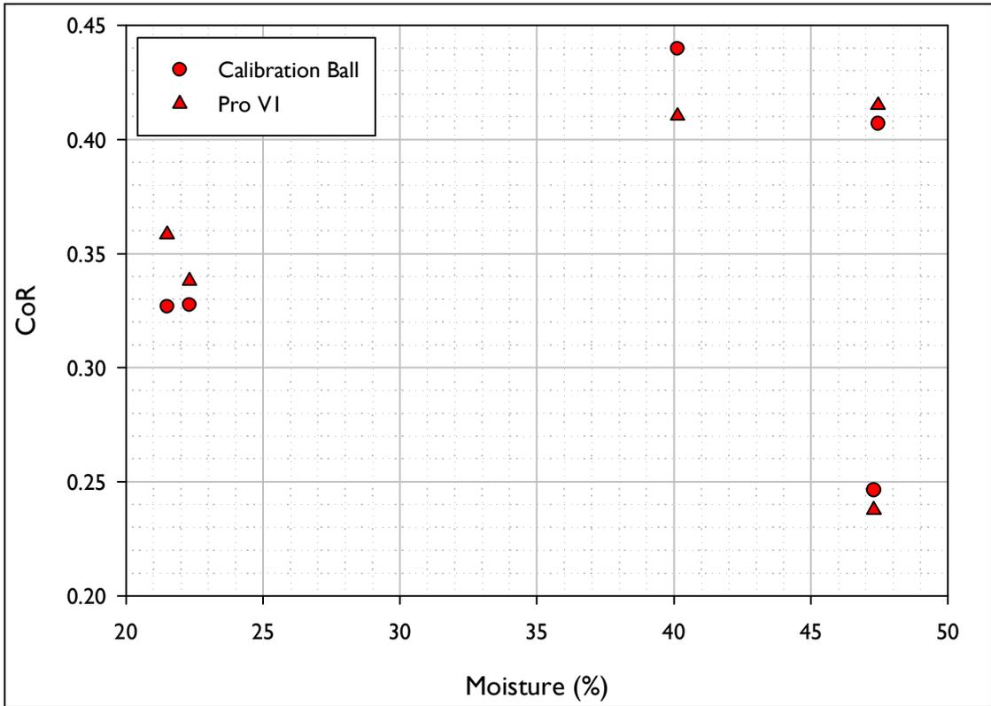
Figure C.5. Vertical Coefficient of Restitution (CoR) vs. Moisture for the shots fired using the inbound conditions akin to those for a Driver.
