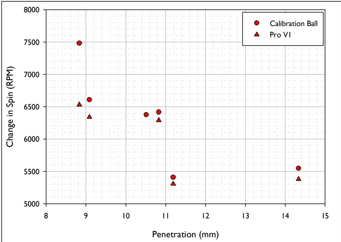
Figure D.3. Change in Spin vs. Penetration for the shots fired using the inbound conditions akin to those for a 5 Iron.
