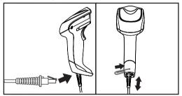
**Host Connection:** The WDI4600 plugs directly into the host device as shown in Figure 2. The power can also be supplied through an external power supply via the Interface Cable supplied with a power jack.
