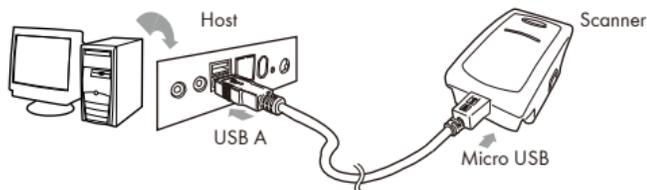
1. Flip open the micro USB port on the scanner.
