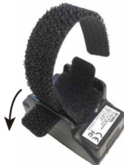
4. Remove the whole Velcro strap from the scanner by pulling the long end.
