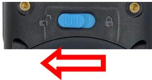
2. Grab the battery cover from the two recesses and lift gently upward to remove it. Remove the battery by pulling the pull tab.
