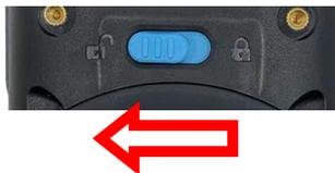
3. Insert the battery cover up to 45 degrees (45°), from bottom to top. Press the battery cover down to secure in place and then slide the battery release latch to the locked position.
