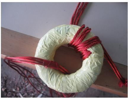
Inductor after spraying with transformer varnish. It is recommended to use a dip procedure for this step instead of spraying.
