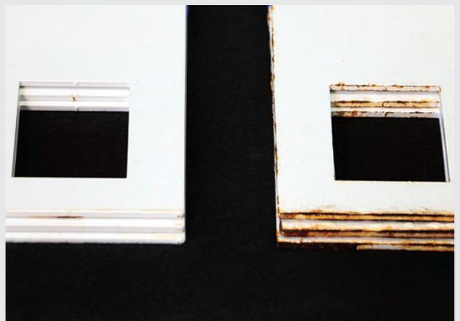
This image of laser-cut edges highlights the edge corrosion performance of a standard DTM powder coating (3 panels on the right) versus PPG's High Edge powder (3 panels on the left) after 40 cycles of cyclic corrosion testing as per SAE J2334.
