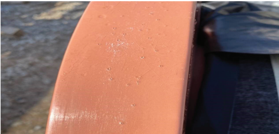
Spider veining/bubbling in past two-coat polyester-based powder system
