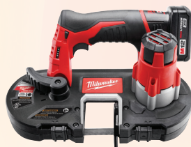
M12™ Sub-Compact Band Saw Cuts through 3/4" EMT in only 3 seconds. 1-5/8" x 1-5/8" cut capacity. Includes: 18 TPI metal cutting blade, M12™ REDLITHIUM XC high capacity battery, M12™ Lithium-Ion battery charger, variable speed trigger and carrying case.
