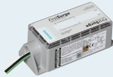
FirstSurge Protective Device Rated 120/240V, split phase (up to 400A) at 50/60Hz, surge spike capacity 60kA, less than 1 nanosecond response time, NEMA 4X enclosure. # SIEFS060
