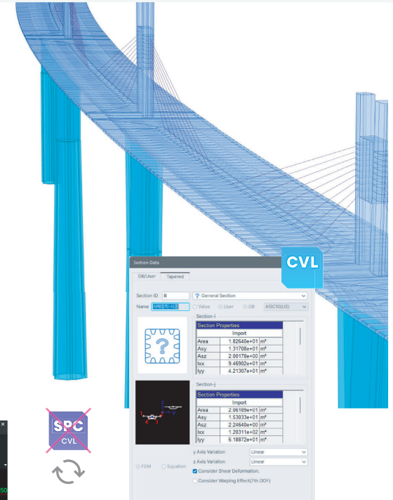
Creation of cross-sections without information loss through automatically calculated properties in CAD
