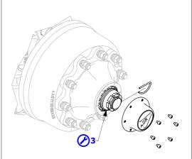
3. Bearing gap check (Teknoax version with screw-in hub cap).
