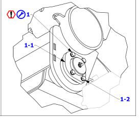
2 - Check oscillating arm articulation nut torque.
