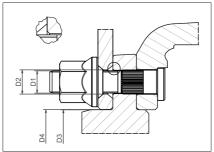
5. Single wheel with conic nut
