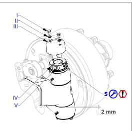
Torque instructions for the regulation nut IV and lock screw V
