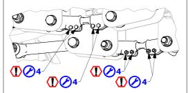
5 – Leaf spring non-slip screw torque check.
