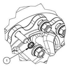
Wheel mounting with centring on hub can be facilitated by the introduction, at least in two columns, of the indicated centring rings, reference 1 in the illustration. This is useful especially when mounting twin wheels since the disc offset could make hub positioning problematic.
