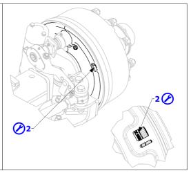
3. Bearing gap check (version with press-in hub cap)
