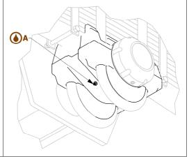
2 - Leaf spring anchoring to the central oscillating support.
