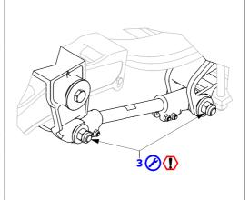
4 – End terminal screw torque check on axle reaction rods
