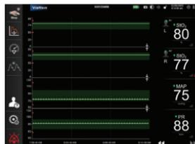
Parameter tiles with the alarm silence icon in the bottom right corner indicate LED and audible alerts are silenced until alarm silence timer ends.
