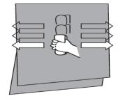
Using a felt tip or flexible nylon squeegee, holding it at a slight upward angle and slightly turned from the center position, use even firm strokes starting at the center top working your way to the outer edges and continuing downward from the center, again to the outer edges.
