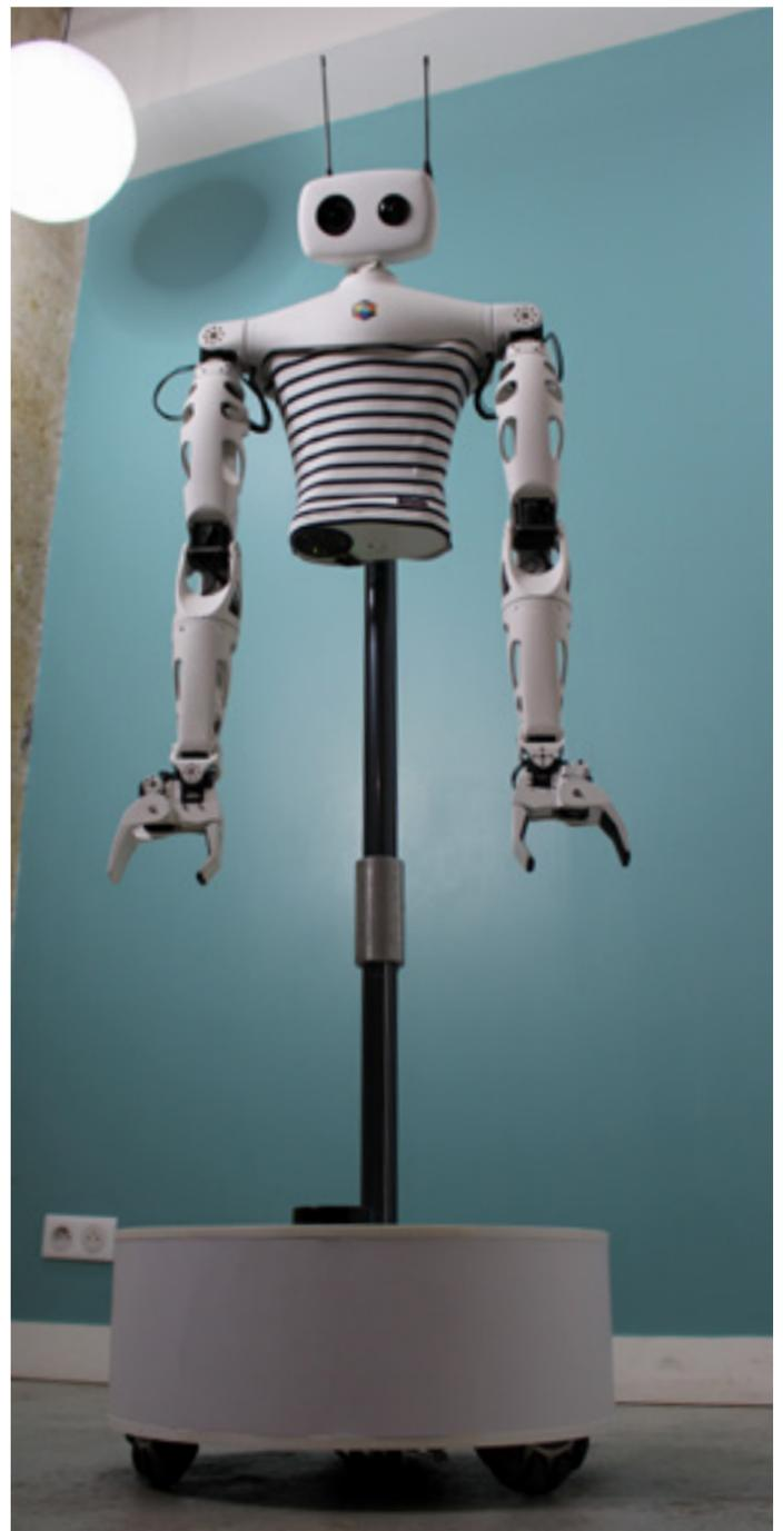
At CES 2020 we introduced Reachy, our open source humanoid robot, to the world. Back then, Reachy was already able to run on autonomous applications thanks to a full Python SDK providing a unified API to simply control the robot locally.
