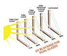
NOTE: Tested units include argon. The laminate has 1/4" inner pane. Based on Lawrence Berkeley Lab (LBL) Window 5.2 © 2003 analysis for classical UV transmission data.
