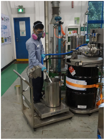
Our aerospace facility in Suzhou, China, eliminated 4,800 one-gallon cans annually by using a 55-gallon drum in the coating color-matching process.
