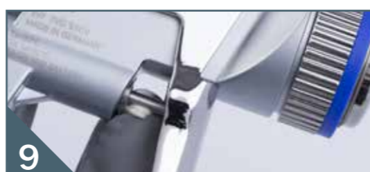
6 Grease and insert paint needle spring
