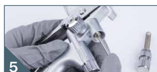
2 Hand-tighten fluid tip with the ring spanner
