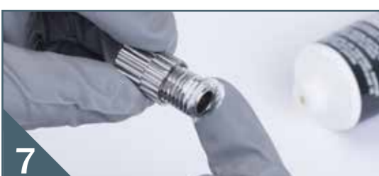
4 Grease paint needle around the needle packing area
