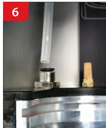
Secure the line to the inside connector on the filling machine.
