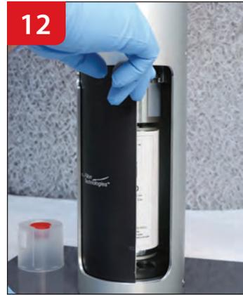
12 Open door; Rotate machine's turntable clockwise; Remove can.
