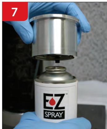
Insert metal cylinder cup on
