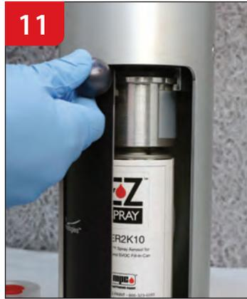
11 Close machine's door to initiate aerosol filling (about 3-6 seconds).
