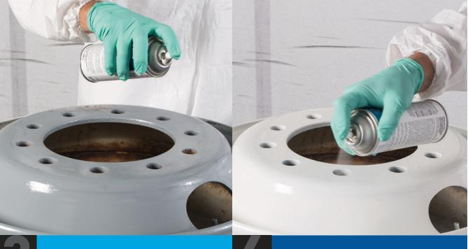
Apply 2 double wet coats of CPC-SP8150 gray primer. Allow to flash for 15 minutes between coats.
