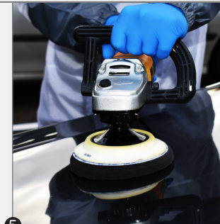
5 Action: Polish compounded surrounding area. Use: Polarshine 5 and Black Dotted 150mm pad. Note: For use on dark colours.
