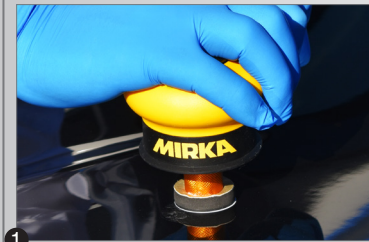
1 Action: Sand dirt nib. Use: Machine and grit SR7 then SR5 disc
