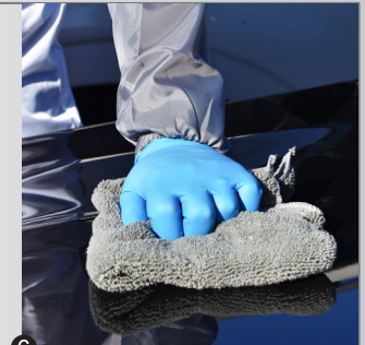
6 Action: Waxed polished area. Use: Polarshine Liquid Nano wax with microfibre cloth.
