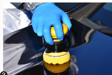
3 Action: Compound sanded area. Use: Polarshine 35 & 85mm Yellow Waffle Pad
