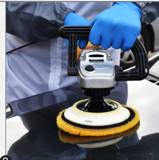
3 Action: Compound sanded area. Use: Polarshine 35 and Lambswol 150mm pad.
