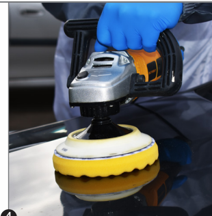
4 Action: Compound sanded area. Use: Polarshine 15 and Yellow Waffle 150mm pad.
