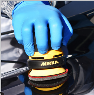
1 Action: Sand defects. Use: Use grit P1200 or P1500.
