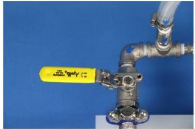
Figure 13: Handle Position to Discontinue the Flow of Air into the System
