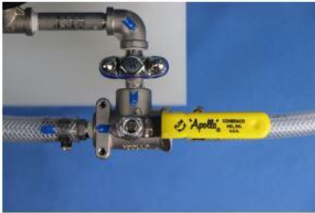
Figure 13: Handle Position to Discontinue the Flow of Air into the System
