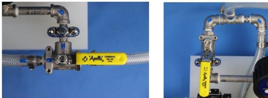
Figure 7: Handle Position: Three-way valve to allow air to flow (left) and Ball valve in open position (right)
