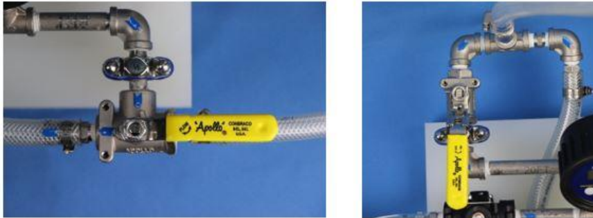
Figure 15: Handle Position to Allow for Flow of Air to Bypass Pressure Pot
