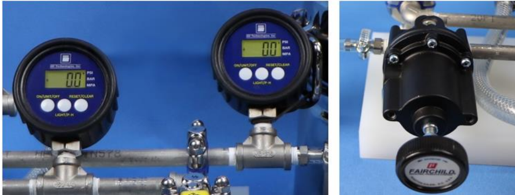
Figure 8: Pressure Gauge and Pressure Regulator
