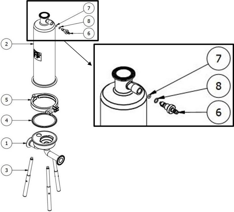
Figure 1: Exploded View of a Single Element Housing
