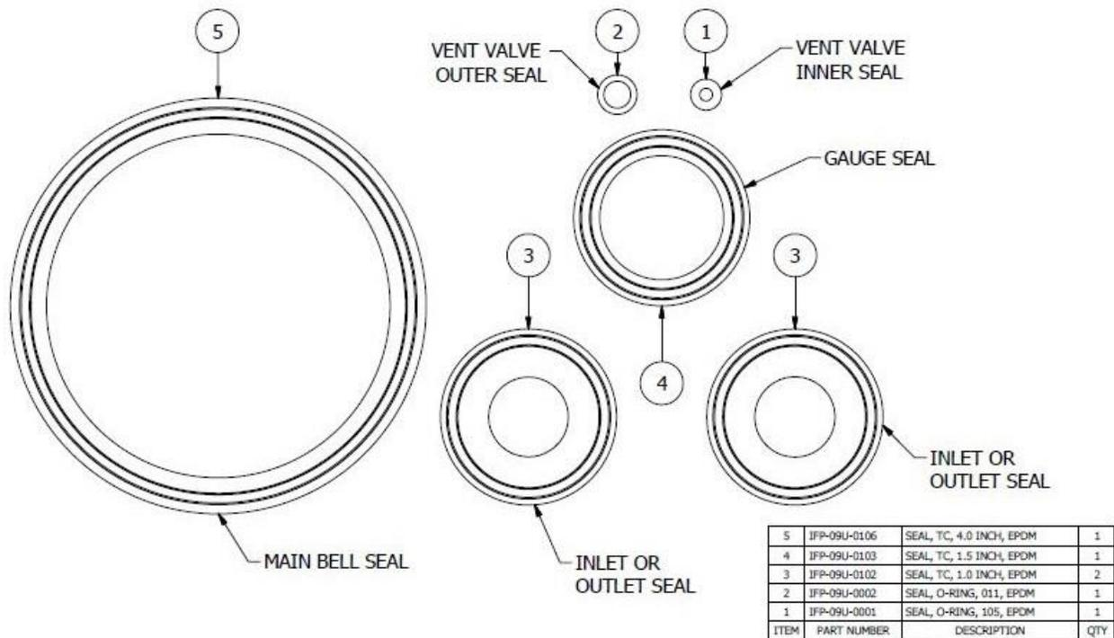
Figure 2: Example of Typical Seal Kit Contents
