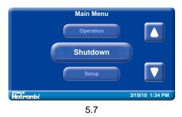
Press the "Shutdown" menu to exit The Fusion<sup>™</sup>. (5.7, 5.8)
