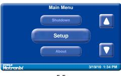
The "Setup" Menu selection screen provides additional system setup functions not accessible from the Main Menu. Those functions are: Presets, Display, Auto On/Off, and Main Menu. (5.5, 5.6)
