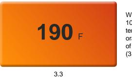
When the heat platen is above 100°F (38°C), the current platen temperature is displayed on a orange background as a warning of the current platen temperature. (3.3)
