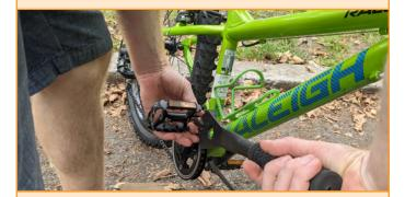
Note: The left pedal is reverse-threaded and thus screws in the opposite direction of the right pedal. That being said, the following applies to both pedals: When standing behind the rear wheel of the bike and looking down on the pedal, turn backwards to loosen and forward to tighten.
