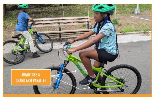
Ideally the crank arm should be parallel to the downtube of the bike, or at about two o'clock. This is called the power pedal position because it gives the rider the most forward propulsion from a stop.
