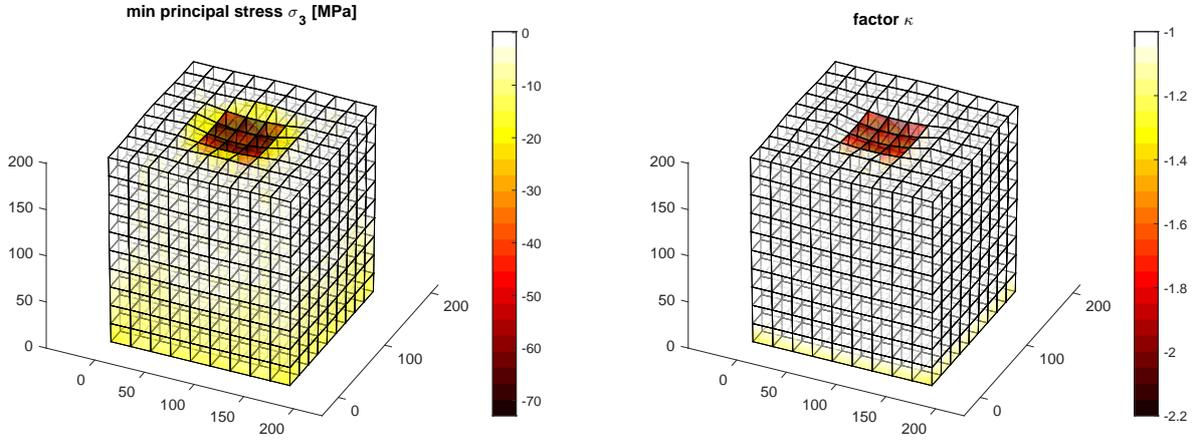
Figure 4: Model results for footing analysis. Left: Minimum principal stress distribution. Right: Factor  $\kappa$  values in locally loaded areas.
