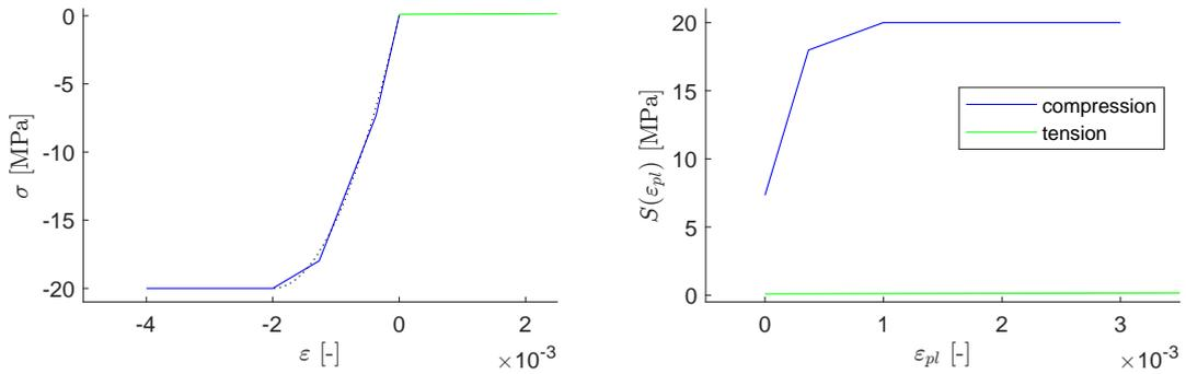
Figure 1: Example of uni-axial material properties: Left: Stress-strain relation, Right: Plastic strain evolution.
