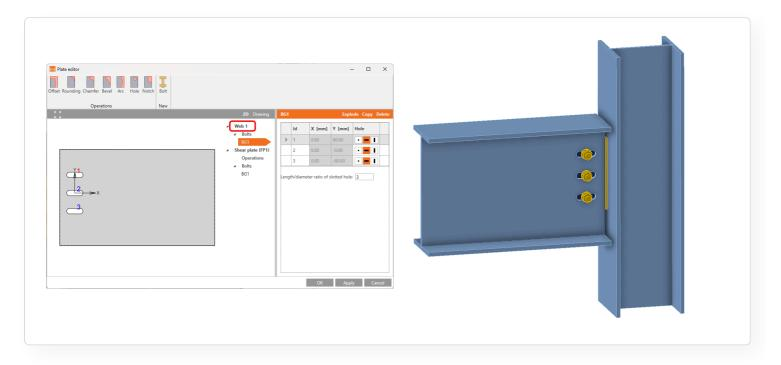
The slotted holes can be assigned to **multiple bolted plates**.
