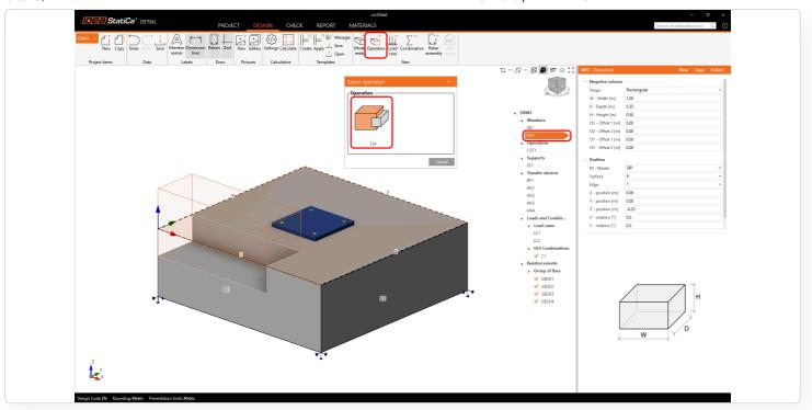
• A Cutting plane works in a similar way. As shown in the following figure, any cut generates new edges and surfaces that can serve as references for placing reinforcement.
