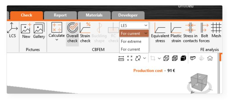
The calculated load effects are available directly in the tree in the 3D scene. Disabled load effects in the Design tab are not shown in the Check tab tree.
