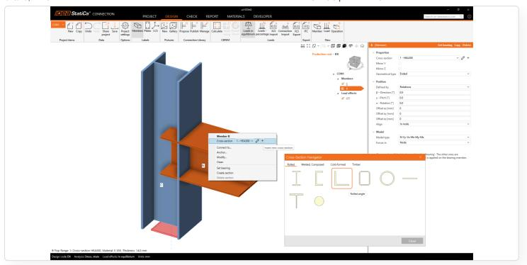
First, the standard section is selected. Using the arrow button, the section can be changed to another one from the library of angles.
