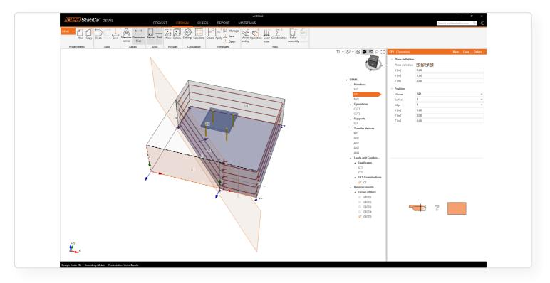
• After the first Cut operation is applied, reinforcement can be referenced to either the original or newly created faces and edges. This is controlled through a new setting in the property grid.
