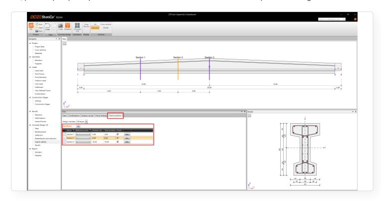
Clicking the **Detailed** button generates an RCS file for the defined sections and selected design situations (LTB analysis has to be completed before opening RCS).
