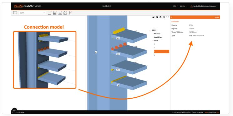
For clarity of outcomes, both values of weld size are displayed at the same time – Leg size and Throat thickness, independent of the units selected.
