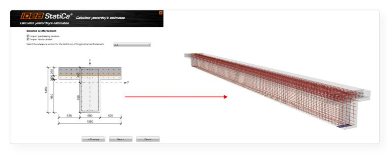
By directly transferring reinforcement details from Beam to Detail, engineers can avoid redundant remodeling, saving both time and effort while maintaining accuracy and consistency across design stages.
