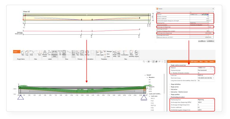
For pre-tensioned strands, straight strand layers in the XZ plane are transferred. The data included for each layer consists of geometry in the XZ plane, stress immediately after release (σ<sub>pm0</sub>), blanked lengths, and the number of strands per layer, ensuring accurate prestressing details in the model. For more information related to pre-tensioning in Detail, including tendon stresses, losses, loading, combinations, etc., read the following article:
