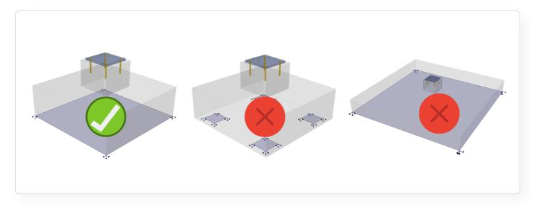
Note: In the case of surface support, failure always occurs at the anchorage area, and punching does not play a role. Only in cases of soils with low stiffness may punching occur, or also in the case of pile caps. For these situations, the software is not yet suitable for use.
