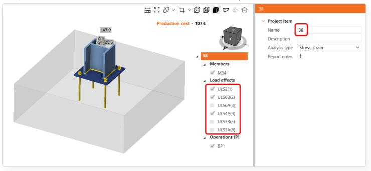
Calculate the group of connections and browse the results for critical load effects. Optimize the design of the reference connection or even reshuffle groups to finish with the best result.
