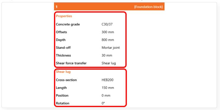
If the Shear force transfer is set to 'Shear lug', these parameters are also provided.
