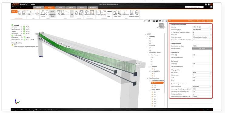
For long-term service combinations, an estimate of long-term losses due to shrinkage and relaxation must be provided as a percentage.
