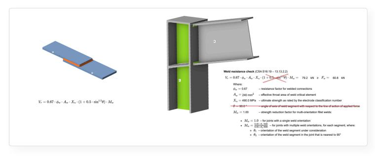
This also affects the calculation of weld strength for Autodesign of welds and applies to all code versions of CSA (also S16-14).
