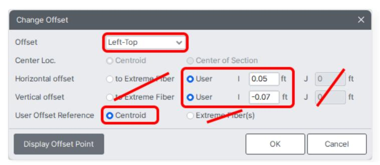
**Note:** Because of the coordinate system orientation used, the eccentricity value sign can be inversed when imported from MIDAS to Checkbot, but the real position, as shown in the 3D model, is correct.
