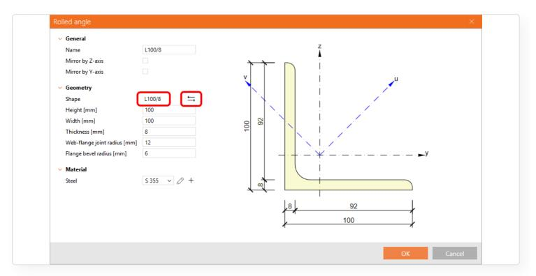
When some parameters are changed (the thickness of the standard section, etc.), the section becomes custom.
