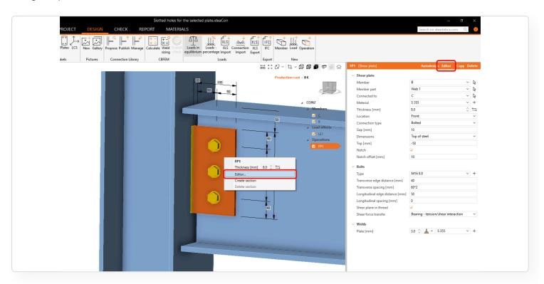
In the plate Editor of the plate containing the bolt, there is a list of all the plates that are connected by selected bolts. In the list, you can define, on which plate the holes will be changed to slotted.
