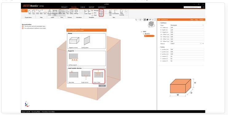
The Cast-in plate allows for welded reinforcement in three shapes: Straight, L-shape, and U-shape.
