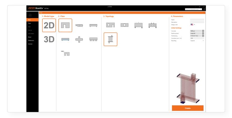
The existing classes include templates for walking columns, deep beams, deep beams with openings for walls, and coupling beams for beam cut-offs. Additionally, there are classes such as whole beams with a total of ten templates, a foundation class with three templates, and a prestressed beam class with five templates.
