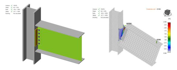
Figure C.2: IDEA StatiCa force applied on bolts in Test No. 5
