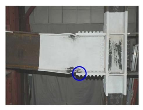
Figure 3.7: Fracture location (Sato et al., 2007)
