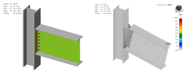
Figure C.12: IDEA StatiCa force applied on bolts in Model 4
