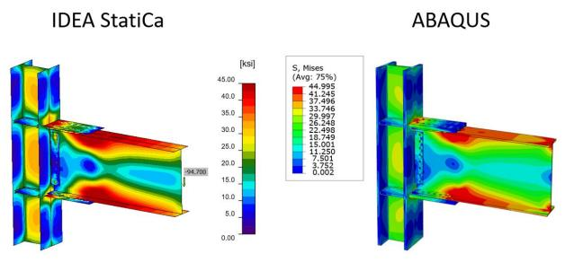
Figure 3.12: Comparison of the predicted von-Mises stress between IDEA StatiCa and ABAQUS
