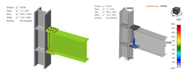
Figure K.10: IDEA StatiCa Model 9 and stress in contact distribution (LRFD)
