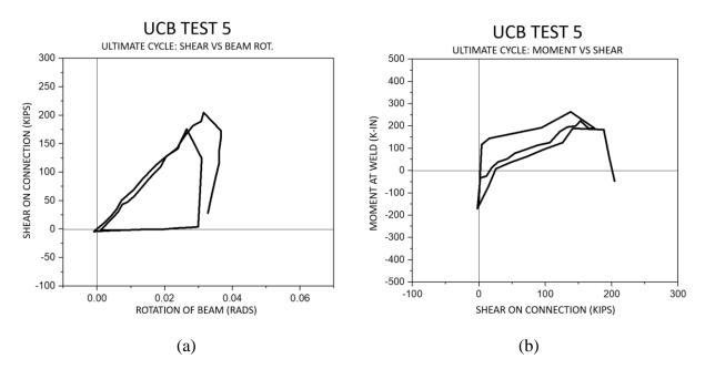
*Figure 1.3: Test specimen No. 5: a) measured shear on connection-rotation of beam relationship, and b) moment at weld-shear on connection relationship*
