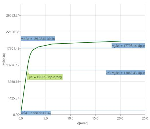
Figure 3.9: Moment-rotation relationship for Test No. BFP (IDEA StatiCa)
