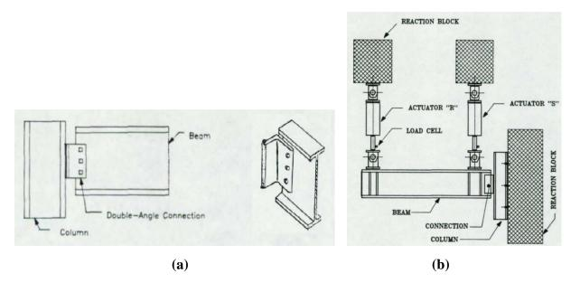
*Figure 1.1: (a) Double angle connection specimens, and (b) test set-up (McMullin and Astaneh, 1988)*
