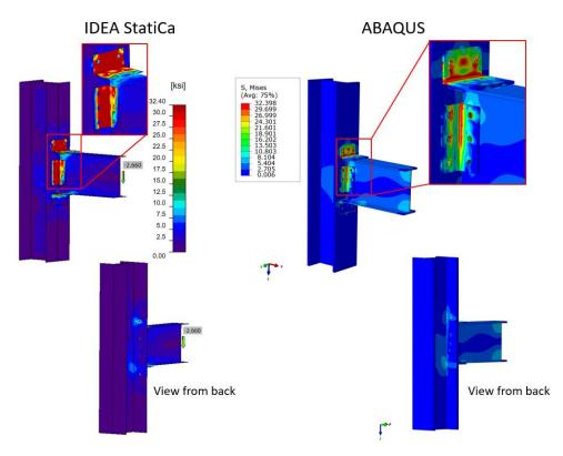
Figure 2.13: Comparison of the predicted von-Mises stress between IDEA StatiCa and ABAQUS
