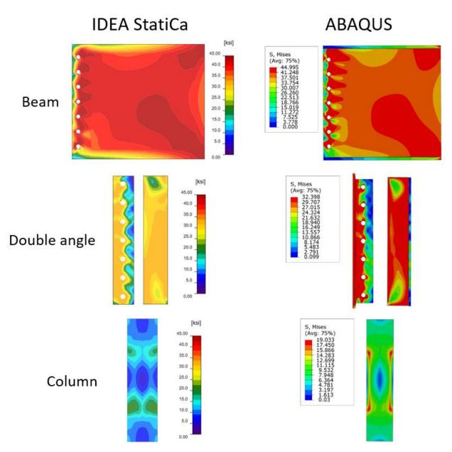
Figure D.2: Comparison of the predicted stress between IDEA StatiCa and ABAQUS for case 2
