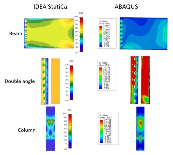
Figure D.1: Comparsion of the predicted stress between IDEA StatiCa and ABAQUS for case 1
