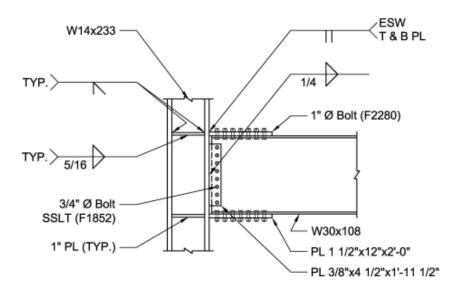
Figure 3.3: Moment connection details for the specimen No. BFP (Sato et al., 2007)
