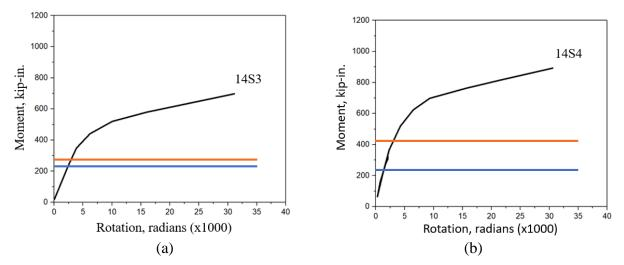
Figure 2.6: Moment-rotation relationship of Test No: a) 14S3 and b) 14S4
