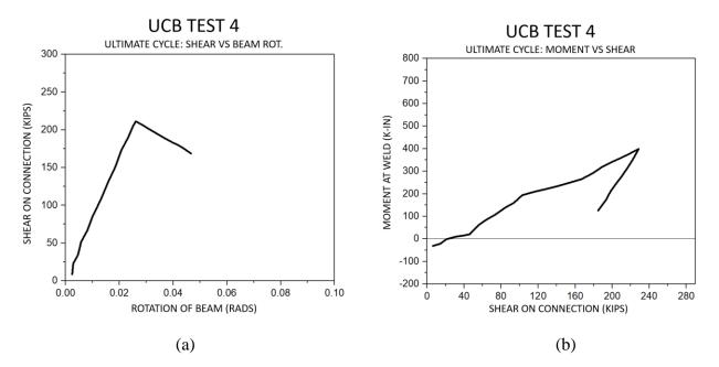
Figure 1.2: Test specimen No. 4: a) measured shear on connection-rotation of beam relationship, and b) moment at weld-shear on connection relationship
