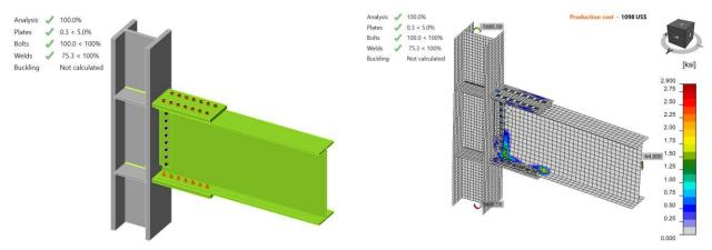
Figure K.8: IDEA StatiCa Model 7 and stress in contact distribution (LRFD)
