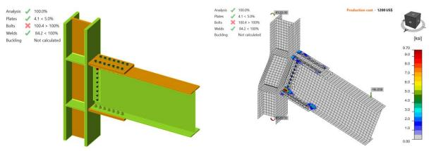
Figure K.2: IDEA StatiCa Model 1 and stress in contact distribution (LRFD)
