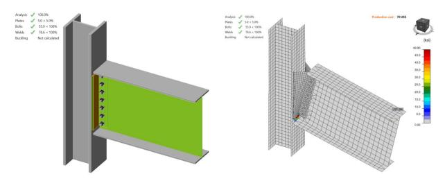
Figure C.9: IDEA StatiCa force applied on bolts in Model 1
