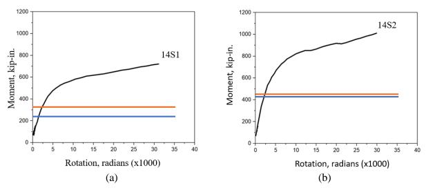
Figure 2.5: Moment-rotation relationship of Test No: a) 14S1 and b) 14S2
