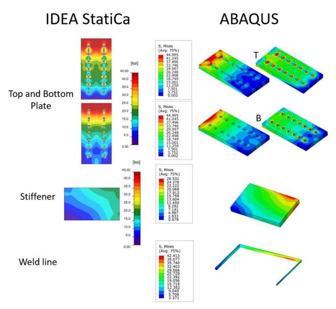
Figure L.1: Predicted stress between IDEA StatiCa and ABAQUS
