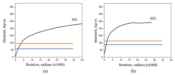
Figure 2.7: Moment-rotation relationship of Test No: a) 8S1 and b) 8S2
