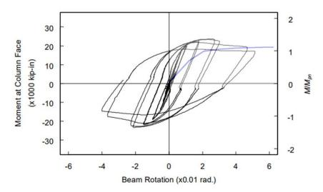
Figure 3.14: Comparison of the moment-rotation relationships of Test No. BFP measured during the experiment and calculated from IDEA StatiCa (blue line)
