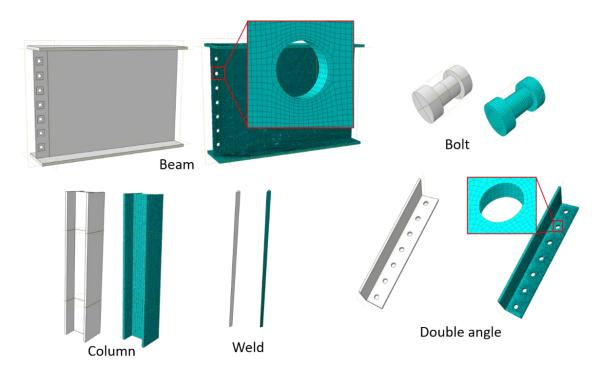
Figure 1.11: ABAQUS model mesh densities
