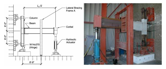
Figure 3.1: Test Setup: (a) schematic; (b) photo (Sato et al., 2007)
