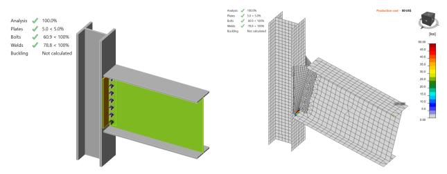
Figure C.14: IDEA StatiCa force applied on bolts in Model 6
