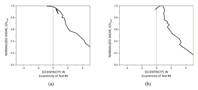
Figure 1.8: (a) Normalized shear-eccentricity of Test No 6, and (b) Normalized shear-eccentricity of Test No 9 (McMullin and Astaneh, 1988)
