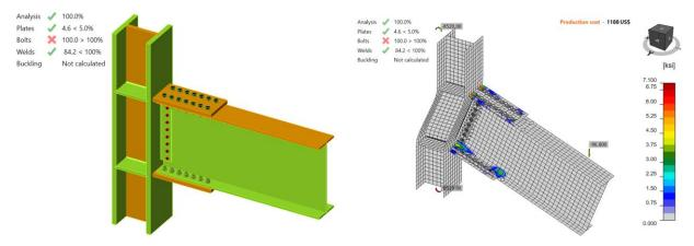
Figure K.3: IDEA StatiCa Model 2 and stress in contact distribution (LRFD)
