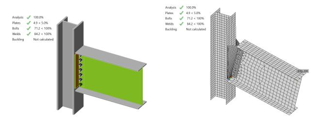
Figure C.13: IDEA StatiCa force applied on bolts in Model 5
