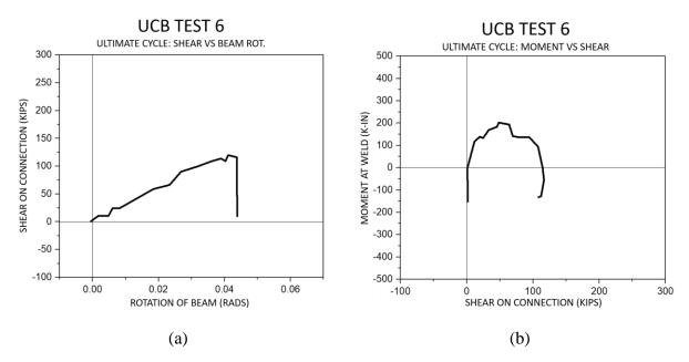
*Figure 1.4: Test specimen No. 6: a) measured shear on connection-rotation of beam relationship, and b) moment at weld-shear on connection relationship*
