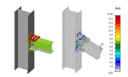
Figure G.7: IDEA StatiCa Test No. 8S3 (LRFD)
