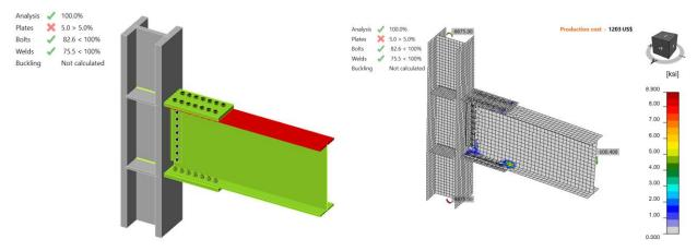
Figure K.6: IDEA StatiCa Model 5 and stress in contact distribution (LRFD)
