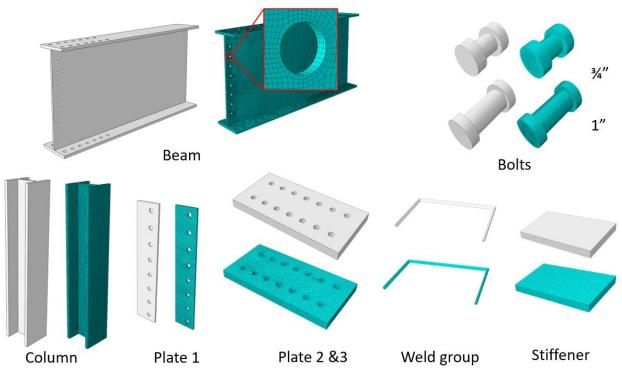
Figure 3.11: ABAQUS model mesh densities
