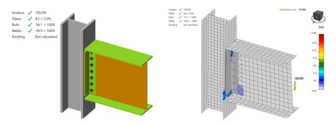
Figure C.16: IDEA StatiCa force applied on welding in Model 2
