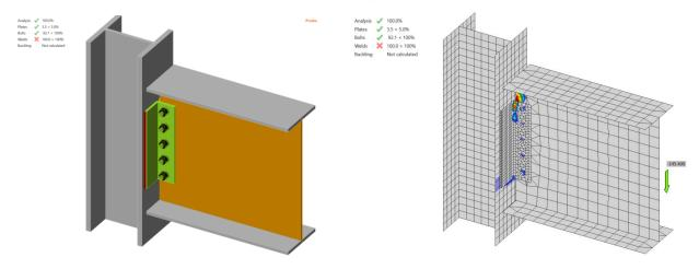
Figure C.6: IDEA StatiCa force applied on welding in Test No. 5
