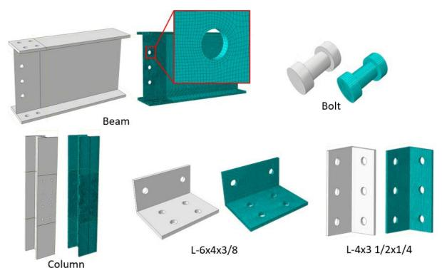
Figure 2.12: ABAQUS model mesh densities
