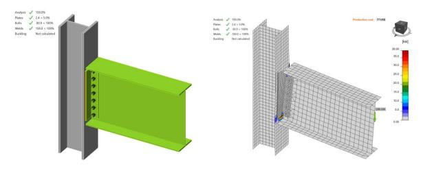
Figure C.10: IDEA StatiCa force applied on bolts in Model 2
