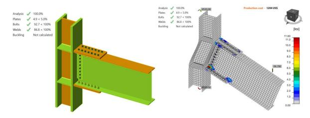
Figure K.1: IDEA StatiCa BFP and stress in contact distribution
