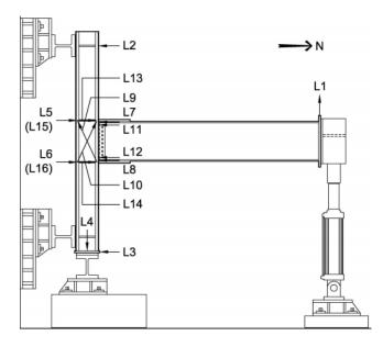
Figure 3.2: Displacement transducer locations (Sato et al., 2007)
