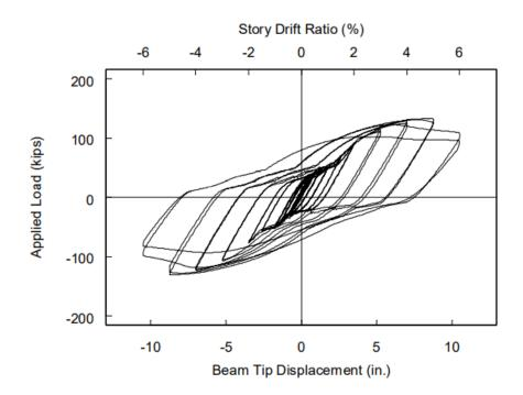
Figure 3.6: Moment at column face-beam rotation (Sato et al., 2007)
