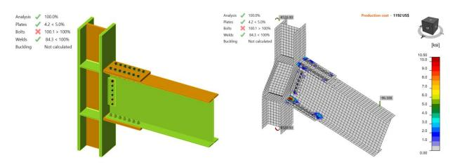
Figure K.4: IDEA StatiCa Model 3 and stress in contact distribution (LRFD)
