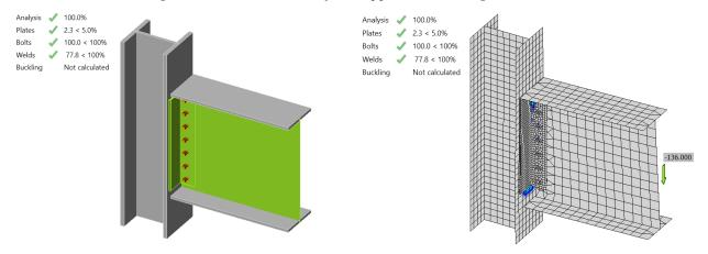
Figure C.17: IDEA StatiCa force applied on welding in Model 3
