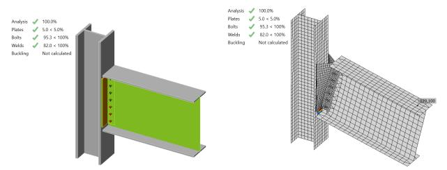
Figure C.11: IDEA StatiCa force applied on bolts in Model 3
