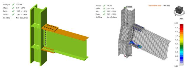
Figure K.9: IDEA StatiCa Model 8 and stress in contact distribution (LRFD)
