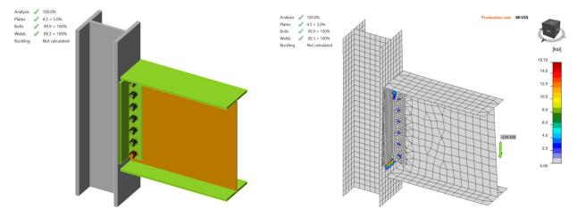
Figure C.20: IDEA StatiCa force applied on welding in Model 6
