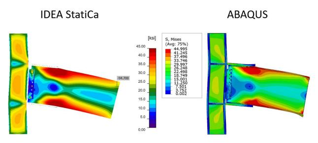
Figure 3.13: Side view comparison between IDEA StatiCa and ABAQUS with deformation scale factor of 20
