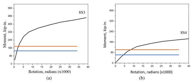
Figure 2.8: Moment-rotation relationship of Test No: a) 8S3, and b) 8S4
