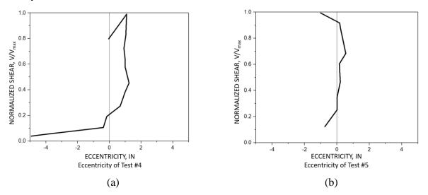
Figure 1.7: (a) Normalized shear-eccentricity of Test No 4, and (b) Normalized shear-eccentricity of Test No 5 (McMullin and Astaneh, 1988)
