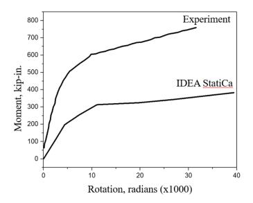
Figure 2.16: Comparison of the moment-rotation relationships of Test No. 14S1 measured during the experiment and calculated from IDEA StatiCa
