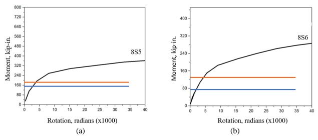
Figure 2.9: Moment-rotation relationship of Test No: a) 8S5, and b) 8S6
