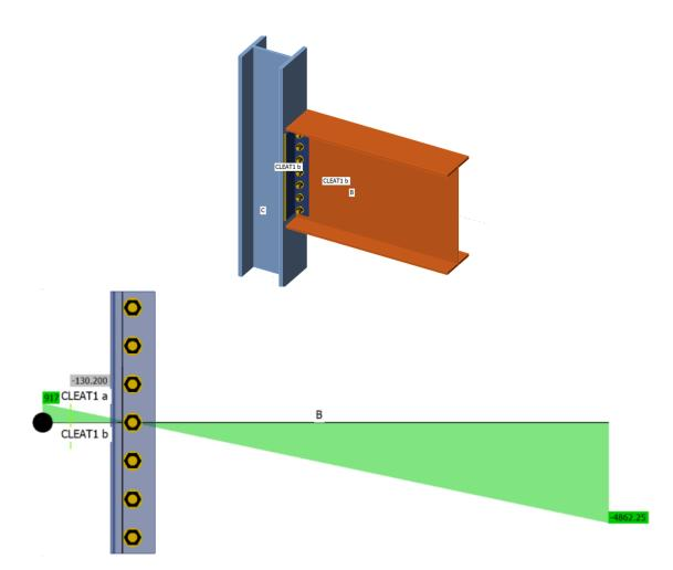
Figure 1.9: IDEA StatiCa model setup (top) and the wireframe model in bottom for the double angle connection specimen, Test No 4 (force applied on the centroid of the bolts group)
