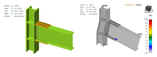
Figure K.7: IDEA StatiCa Model 6 and stress in contact distribution (LRFD)
