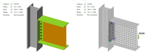
Figure C.15: IDEA StatiCa force applied on welding in Model 1
