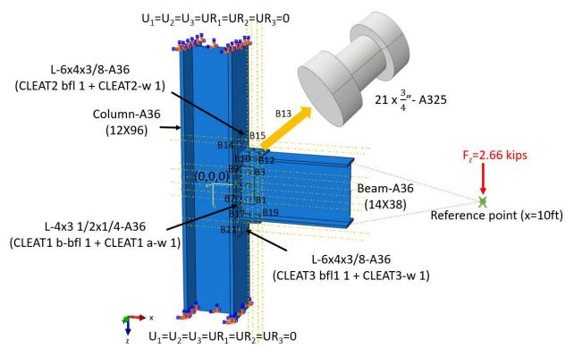
Figure 2.11: Semi-rigid connection model setup in ABAQUS
