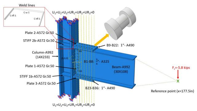
Figure 3.10: Model setup in ABAQUS
