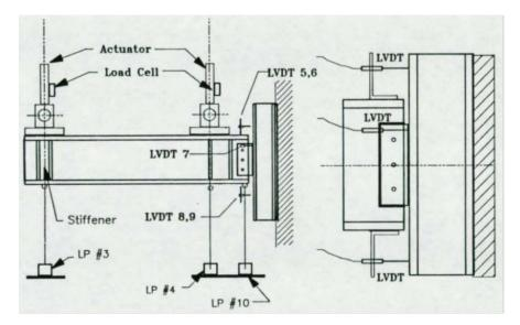
Figure 1.6: Diagram of the instrumentation used during the experiment (McMullin and Astaneh, 1988)
