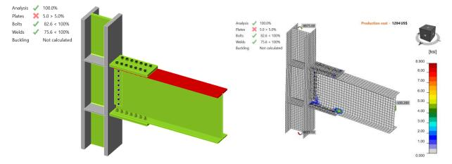
Figure K.5: IDEA StatiCa Model 4 and stress in contact distribution (LRFD)
