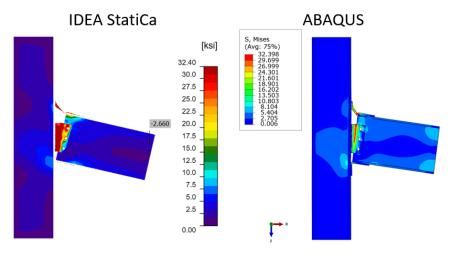
Figure 2.14: Side view comparison between IDEA StatiCa and ABAQUS with deformation scale factor of ten
