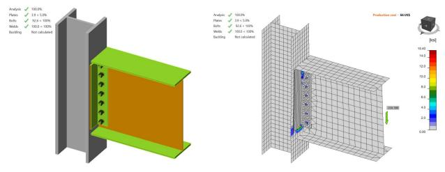
Figure C.18: IDEA StatiCa force applied on welding in Model 4
