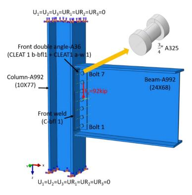
Figure 1.10: Model setup in ABAQUS
