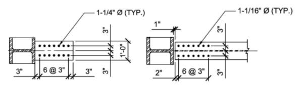
Figure 3.4: Bolt schedule details for the specimen No. BFP: (a) flange plate; and (b) beam flange (Sato et al., 2007)
