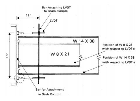
Figure 2.2: Measurements of horizontal displacements using the LVDT apparatus
