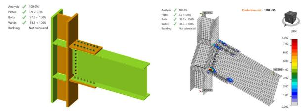
Figure K.11: IDEA StatiCa BFP and stress in contact distribution (ASD)
