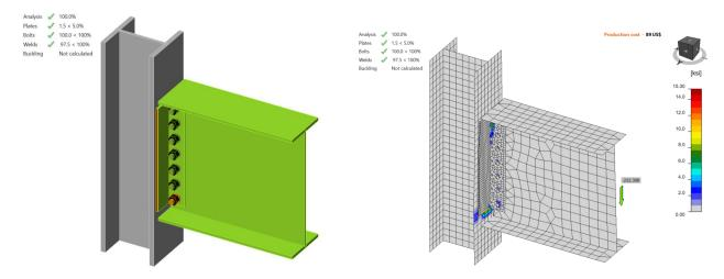
Figure C.19: IDEA StatiCa force applied on welding in Model 5
