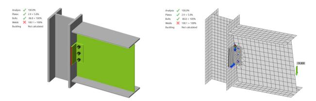
Figure C.7: IDEA StatiCa force applied on welding in Test No. 6
