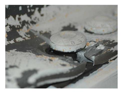
Figure 3.8: Beam bottom flange net section fracture on 2nd cycle at +6% drift
