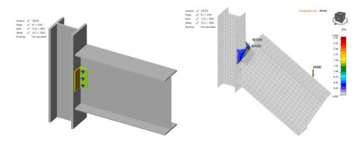
Figure C.3: IDEA StatiCa force applied on bolts in Test No. 6
