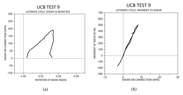
*Figure 1.5: Test specimen No. 9: a) measured shear on connection-rotation of beam relationship, and b) moment at weld-shear on connection relationship*
