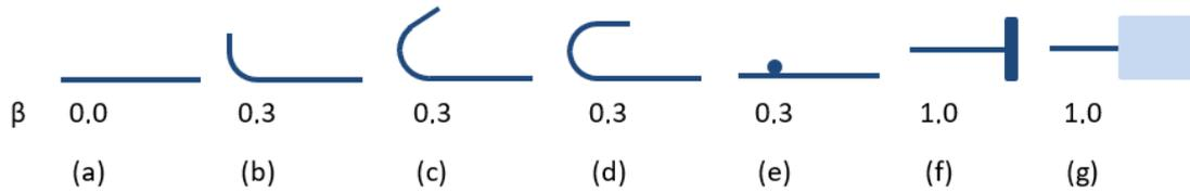
**Fig. 17** Available anchorage types and respective anchorage coefficients for longitudinal reinforcing bars in the CSFM: (a) straight bar; (b) bend; (c) hook; (d) loop; (e) welded transverse bar; (f) perfect bond; (g) continuous bar.
