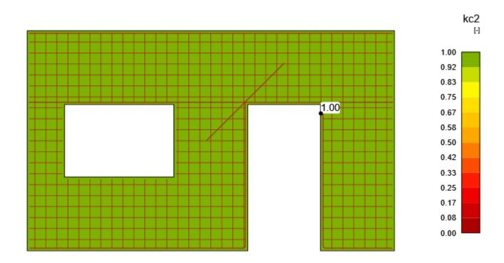
Reinforcement strain/limit strain ratio -  $\epsilon_s/\epsilon_{s,lim}$  [%]
